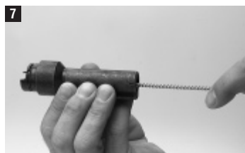
7 Interior del guía-clavos
