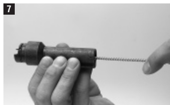
7 Inside of fastener guide
