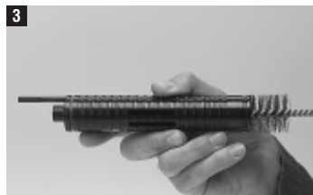
3 Inside of piston guide
