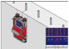
Using the second method, with the aid of the display, the objects are marked at the outside edges of the Hilti PS 1000 X-Scan.
