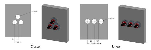
Note: dimensions above relate to  $\emptyset$ 122mm (CFS-SL GA M/L) – using smaller diameters will alter the distances between opening centres.
