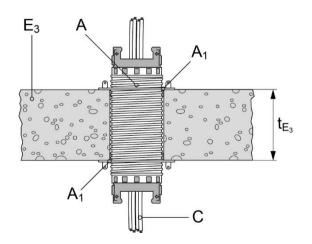
Section – CFS-SL GA M/L in Timber Walls and Floors
