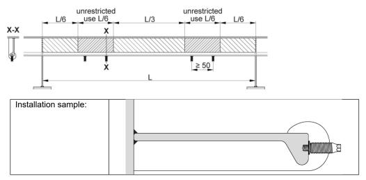
The S-BT fasteners may also be used in the restricted areas based on a case-by-case static investigation.
