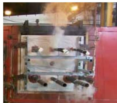
Fire test after seismic impacts
