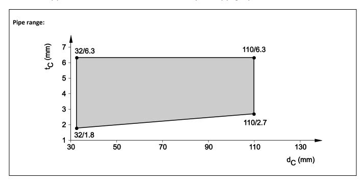
8.6.2.3 PVC pipes acc. EN 1452-1, EN 1329-1, EN 1453-1, EN 1566-1 and EN ISO 15493, in shaft wall system A, pipe group 1, EI 90 - U/U
