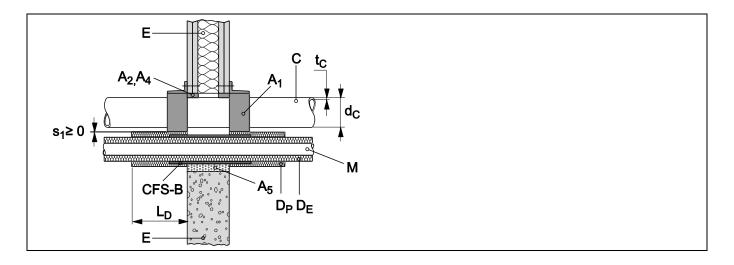
8.3.2.23.2 Pipes in flexible wall (t<sub>E</sub> ≥ 100 mm), pipe group 1, El 90, zero distance between CFS-C EL collar and CFS-B, wrapped around an elastomeric foamed thermal insulation on metal pipe
