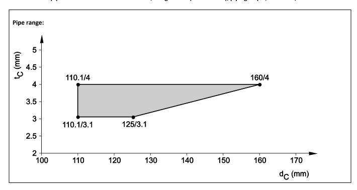
8.5.2.21 PVC pipes acc. EN 1452-1, EN 1453-1, EN 1566-1, EN 1329-1 and EN ISO 15493, in rigid floor (t<sub>E</sub> ≥ 150 mm), pipe group 2, EI 90 - U/U
