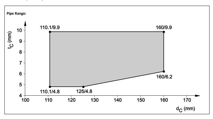
8.4.2.22 ABS pipes acc. EN 1455-1, EN 15493 and SAN+PVC-pipes acc. EN 1565-1, in rigid wall ( $t_E \ge 150$  mm), pipe group 2, EI 120 - U/C
