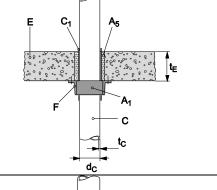
Plastic pipe, penetrating a rigid floor, sealed with Hilti Firestop Collar Endless CFS-C EL. Used gap filler is CFS-S ACR in a thickness of ( $t_{A2} \ge 25$  mm) from the upper surface of the floor only, backfilled with mineral wool.
