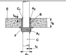
Plastic pipe, penetrating a rigid floor, sealed with Hilti Firestop Collar Endless CFS-C EL. Used gap filler is CFS-S ACR in a thickness of ( $t_{A2} \ge 25$  mm) from both surfaces of the floor, no backfilling is requested.
