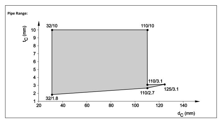
8.3.2.8 PVC pipes acc. EN 1452-1, EN 1329-1, EN 1453-1, EN 1566-1 and EN ISO 15493, in flexible wall ( $t_E \ge 100$  mm), pipe group 1, EI 120 - U/U
