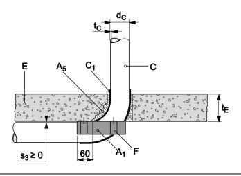
8.5.2.48 PVC pipes acc. EN 1452-1, EN 1329-1, EN 1453-1, EN 1566-1 and EN ISO 15493, in rigid floor (t<sub>E</sub> ≥ 150 mm), pipe group 1, EI 120 - U/U, Pipe Elbow 87°
