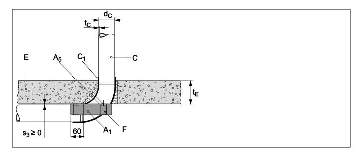
8.5.2.14 PE pipes, non-regulated (Geberit Silent dB20), in rigid floor (t<sub>E</sub> ≥ 150 mm), pipe group 1, EI 120 - U/U straight (90°), pipe coupling
