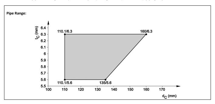
8.5.2.28 PE-X - pipes acc. EN 15875 (Rehau Rautitan flex), insulated, in rigid floor (t<sub>E</sub> ≥ 150 mm), pipe group 1, EI 120 - U/C
