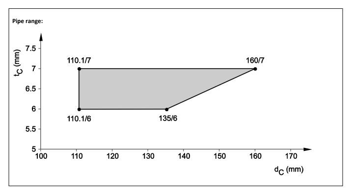
8.5.2.26 PVC pipes acc. EN 1452-1, EN 1329-1, EN 1453-1, EN 1566-1 and EN ISO 15493, in rigid floor (t<sub>E</sub> ≥ 150 mm), pipe group 2, EI 120 - U/C situation
