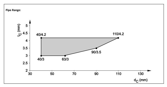
8.3.2.2 ABS- pipes acc. EN 1455, EN 15493 and SAN+PVC-pipes acc. EN 1565-1, in flexible wall, ( $t_E \ge 100$  mm), pipe group 1, EI 90 - U/U
