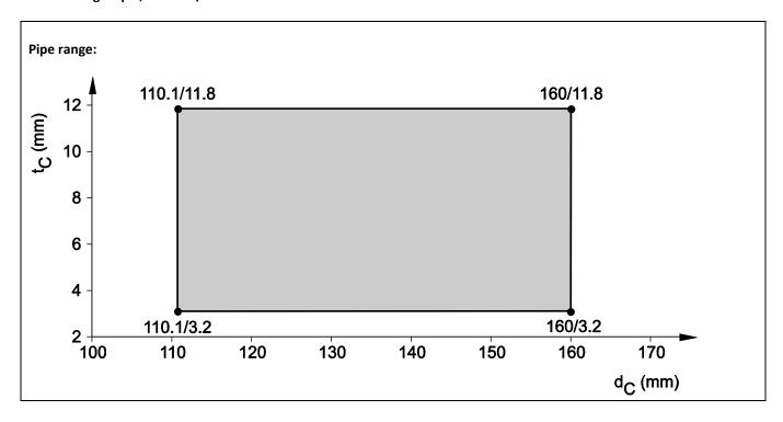
8.5.2.22 PP pipes, non-regulated, in rigid floor (t<sub>E</sub> ≥ 150 mm), pipe group 2, EI 120 - U/U
