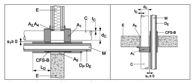
In floor application ( $tR_ER \ge 150$  mm) there is no need for an additional protect insulation DR<sub>P</sub>R.
