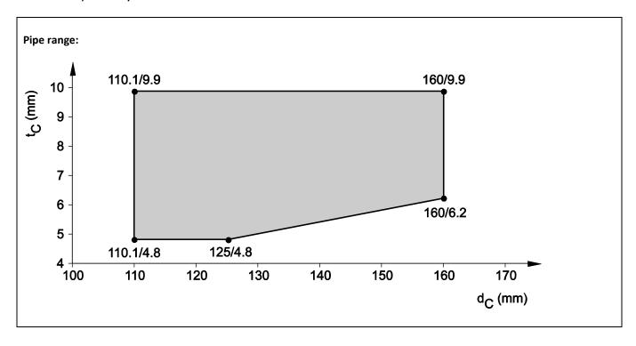
8.5.2.18 PE pipes acc. EN 15494 and EN 12201-2, in rigid floor ( $t_E \ge 150$  mm), pipe group 2, EI 90 - U/U
