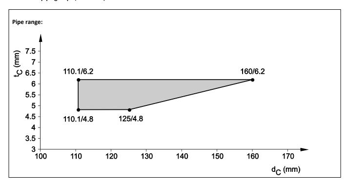
8.5.2.16 ABS pipes acc. EN 1455-1, EN 15493 and SAN+PVC-pipes acc. EN 1565-1, in rigid floor ( $t_E \ge 150$  mm), pipe group 2, EI 120 - U/U
