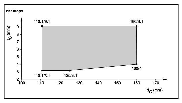
8.4.2.24 PVC pipes acc. EN 1452-1, EN 1329-1, EN 1453-1, EN1566-1 and EN ISO 15493, in rigid wall (t<sub>E</sub> ≥150 mm), pipe group 2, EI 120 - U/U
