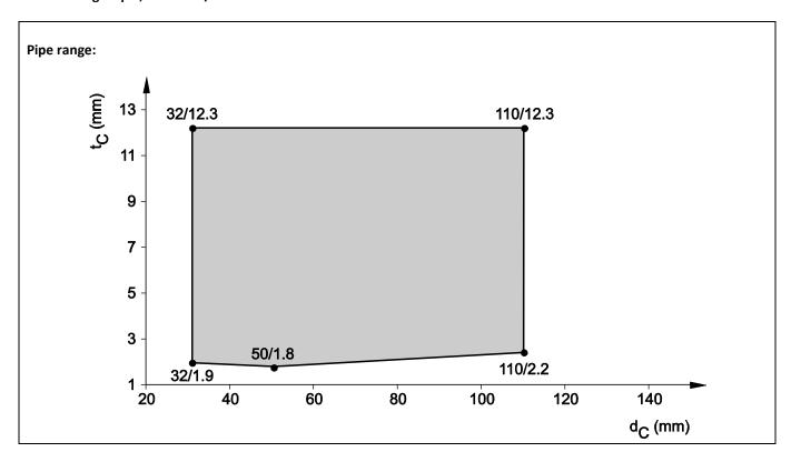
8.5.2.5 PVC pipes acc. EN 1452-1, EN 1329-1, EN 1453-1, EN 1566-1 and EN ISO 15493, in rigid floor (t<sub>E</sub> ≥ 150 mm), pipe group 1, EI 90 - U/U
