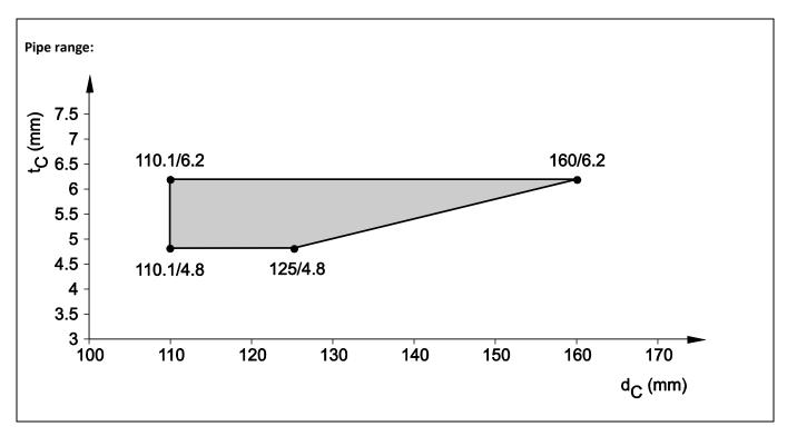
8.5.2.17 ABS pipes acc. EN 1455-1, EN 15493 and SAN+PVC-pipes acc. EN 1565-1, in rigid floor ( $t_E \ge 150$  mm), pipe group 2, EI 60 - U/U
