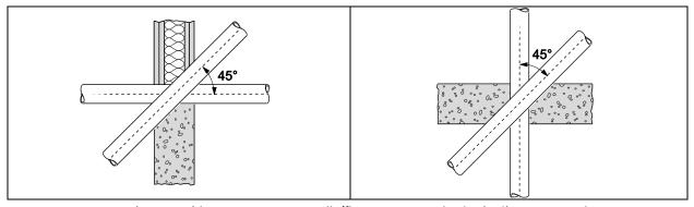
Pipes in pipe group 2 (see 8.2.2) have to penetrate walls/floors in perpendicular (90°) situation only.
