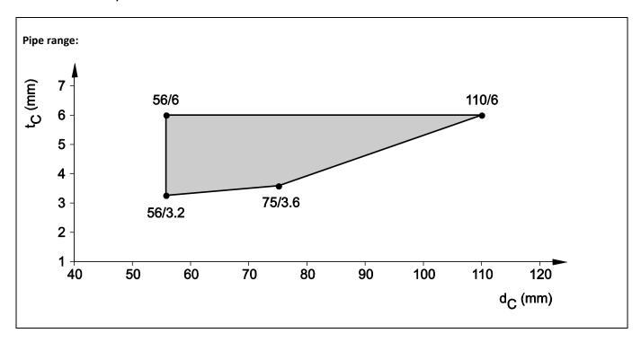
8.6.2.7 ABS pipes acc. EN 1455-1, EN 15493 and SAN+PVC-pipes acc. EN 1565-1, in shaft wall system A, pipe group 1, EI 90 - U/U
