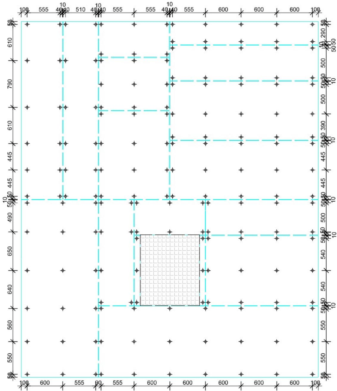
Elevation of revised test wall (wind load tests) showing panel arrangement and panel fixing locations
