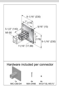
**Material properties** Material Connector and Toothed plate: S235JR - DIN EN10025-2 2005.4 One hand screw, prevail torque hex nut  $f_y = 92.82 \text{ ksi } (640 \frac{N}{mm^2})$   $f_u = 116.03 \text{ ksi } (800 \frac{N}{mm^2})$ Class 8.8 - DIN EN 1993-1-8
