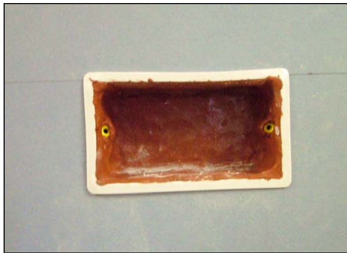
Photograph 1 Putty and wall box installed into the source room side of the partition.
