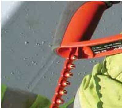
Use Red cartridges for steel. Black cartridges for harder or high strength steel
