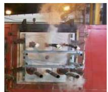
Fire test after seismic impacts
