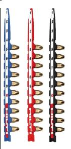
Cartridges 6,8/18 M10 with 10 cartridges per plastic strip for DX 76, DX 76 PTR
