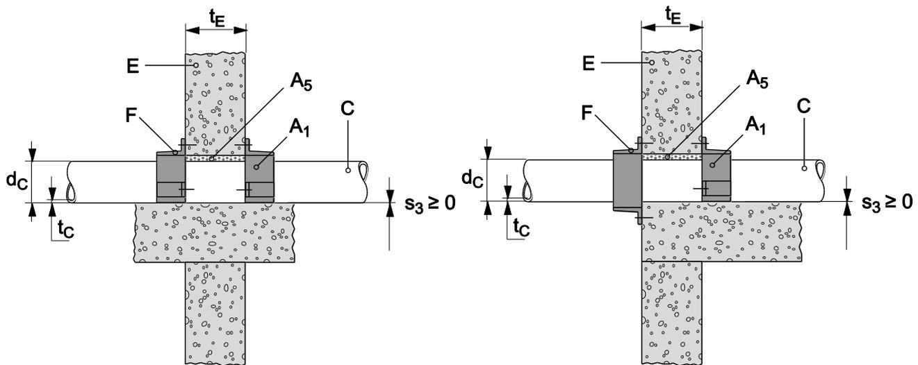
8.4.2.9 **Multiple pipe penetration, covered with foamed elastomeric thermal insulation in rigid wall ( $t_E \geq 100$  mm), pipe group 1, EI 120, U/U + U/C**
