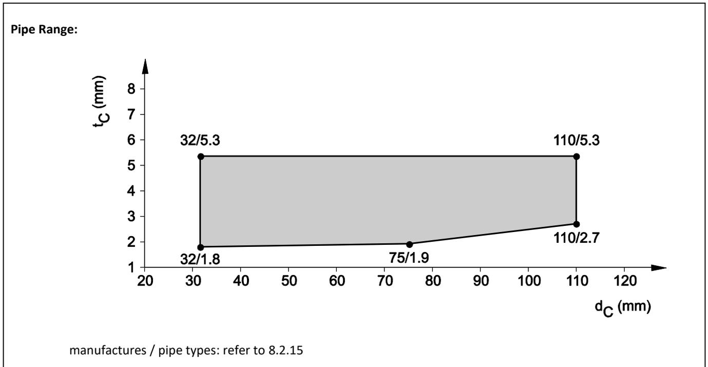
8.3.2.10 PP pipes acc. EN 1451-1, in flexible wall ( $t_E \geq 100$  mm), pipe group 1, EI 120 - U/U
