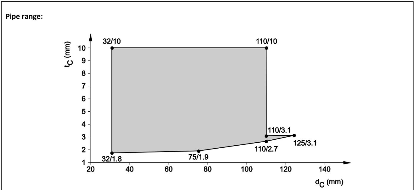
8.5.2.10 PE pipes, non-regulated (Geberit Silent dB20), in rigid floor ( $t_E \geq 150$  mm), pipe group 1, EI 120 - U/U
