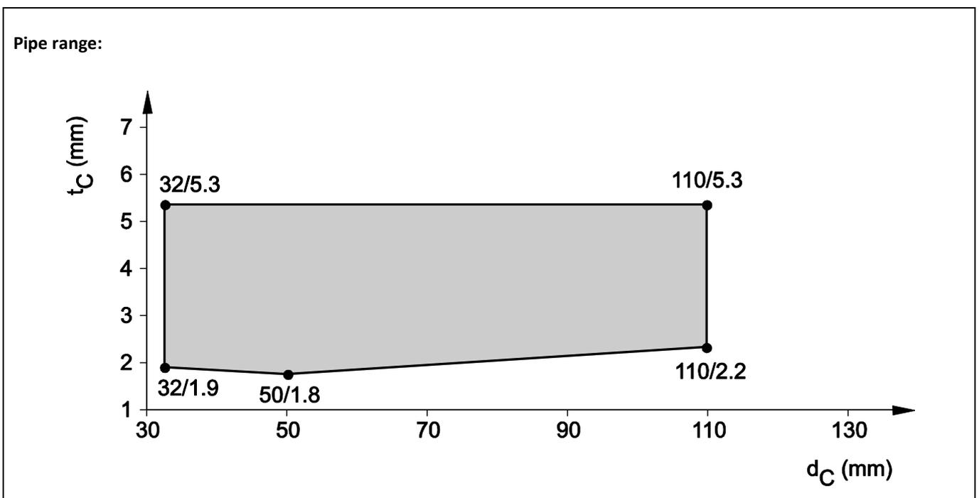
8.6.2.4 PP pipes, non-regulated, in shaft wall system A, pipe group 1, EI 90 - U/U
