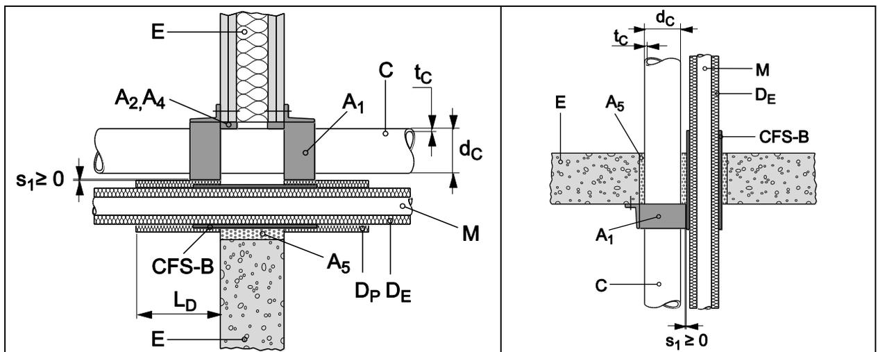
In floor application ( $t_{R,E,R} \geq 150$  mm) there is no need for an additional protect insulation  $DR_{P,R}$ .
