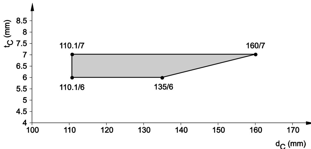
8.4.2.31 PVC- pipes, non-regulated (Friatec Friaphon), in rigid wall ( $t_E \geq 150$  mm), pipe group 2, EI 120 - U/U
