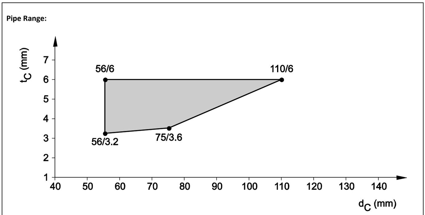
8.3.2.13 PVC- pipes, non-regulated (Friatec Friaphon), in flexible wall ( $t_E \geq 100$  mm), pipe group 1, EI 90 - U/U
