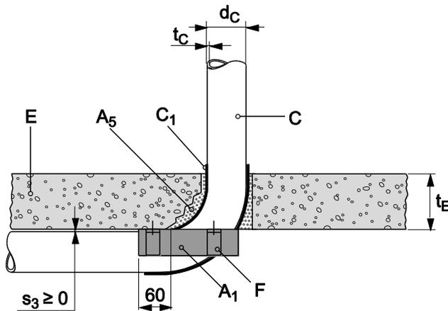
8.5.2.49 **Wavin Tigris PE-X - one pipe in rigid floor ( $t_E \geq 150$  mm), pipe group 1, EI 90 - U/C**
