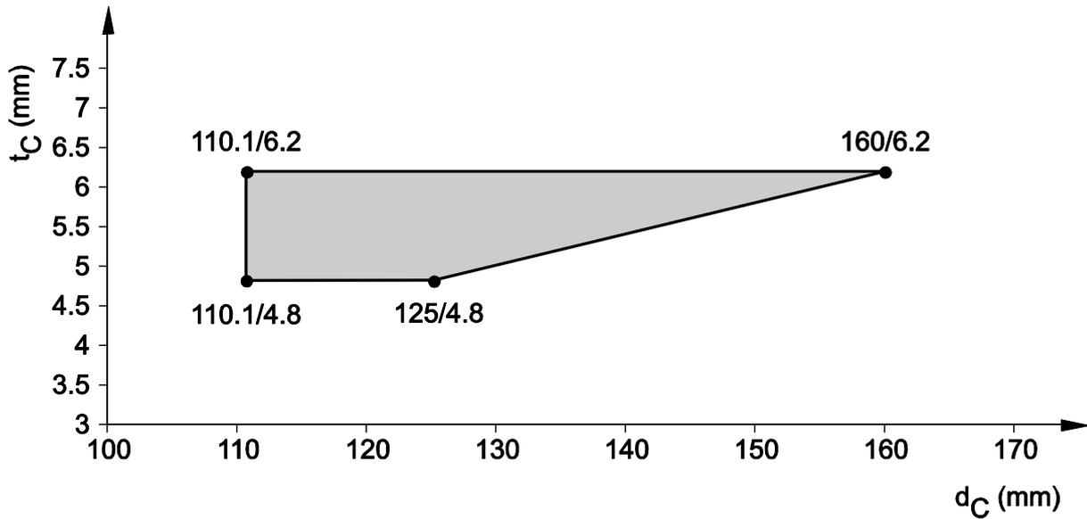
8.4.2.21 ABS pipes acc. EN 1455-1, EN 15493 and SAN+PVC-pipes acc. EN 1565-1, in rigid wall ( $t_E \geq 150$  mm), pipe group 2, EI 90 - U/U
