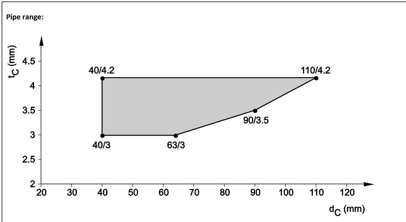
8.6.3.2 PP pipes, non regulated, in shaft wall system B, pipe group 1, EI 90 - U/U
