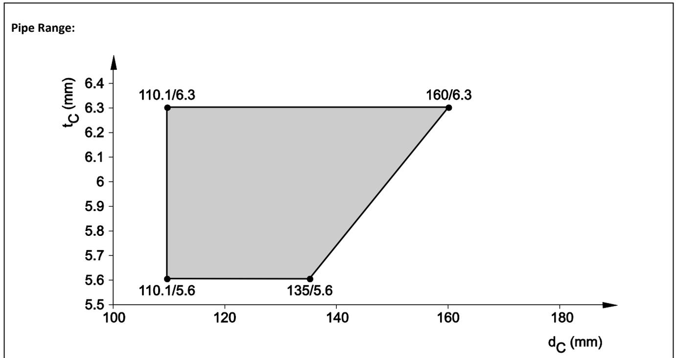
8.4.2.32 Pipes in rigid wall ( $t_E \geq 150$  mm), zero distance collar to collar, pipe group 2, EI 90 - U/U
