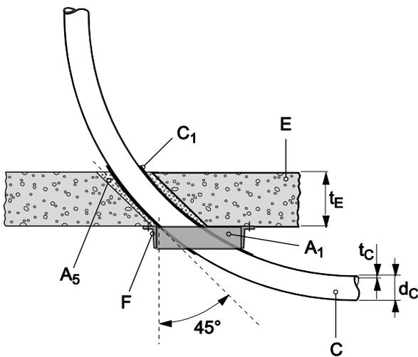
8.5.2.13 **PE pipes, non-regulated (Geberit Silent dB20), in rigid floor ( $t_E \geq 150$  mm), pipe group 1, EI 120 - U/U, straight ( $90^\circ$ ), 2 x  $45^\circ$  elbow pipe connector**
