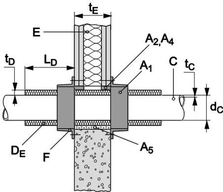
8.3.2.16 PP-R pipe acc. EN 15874 (Aquatherm fusiolen = aquatherm green pipe S), in flexible wall ( $t_E \geq 100$  mm), pipe group 1, EI 120 - U/C
