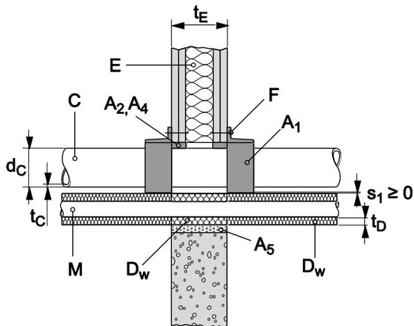
Aluminum composite pipes EI90 U/C
