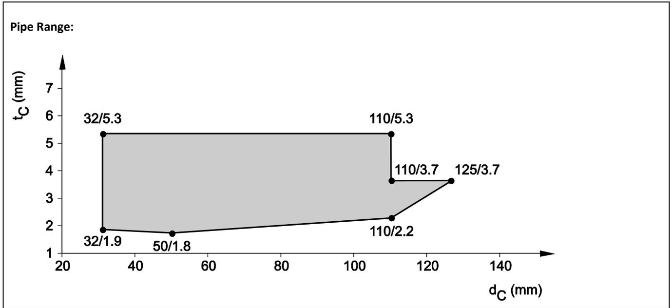
8.4.2.5 PP pipes, non-regulated, in rigid wall ( $t_E \geq 100$  mm), pipe group 1, EI 120 - U/U
