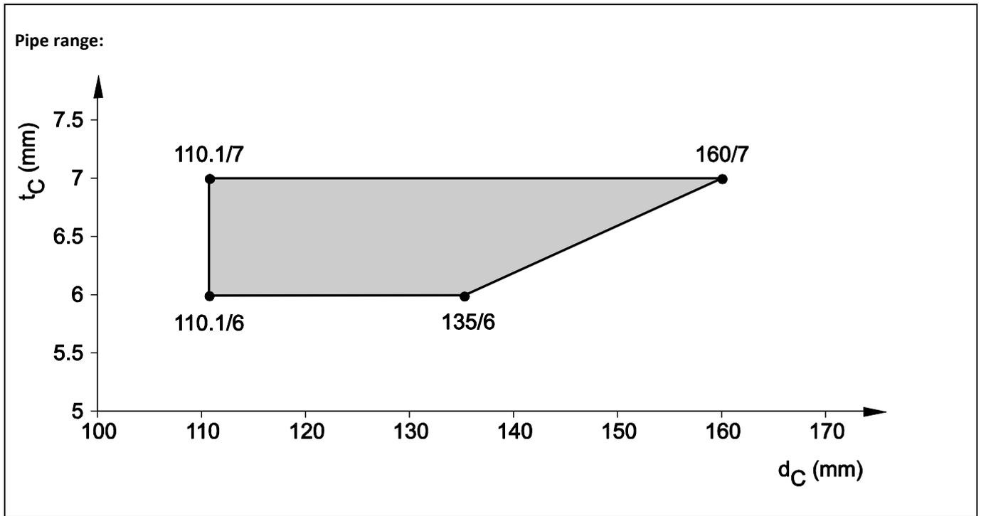
8.5.2.26 PVC pipes acc. EN 1452-1, EN 1329-1, EN 1453-1, EN 1566-1 and EN ISO 15493, in rigid floor ( $t_E \geq 150$  mm), pipe group 2, EI 120 - U/C situation
