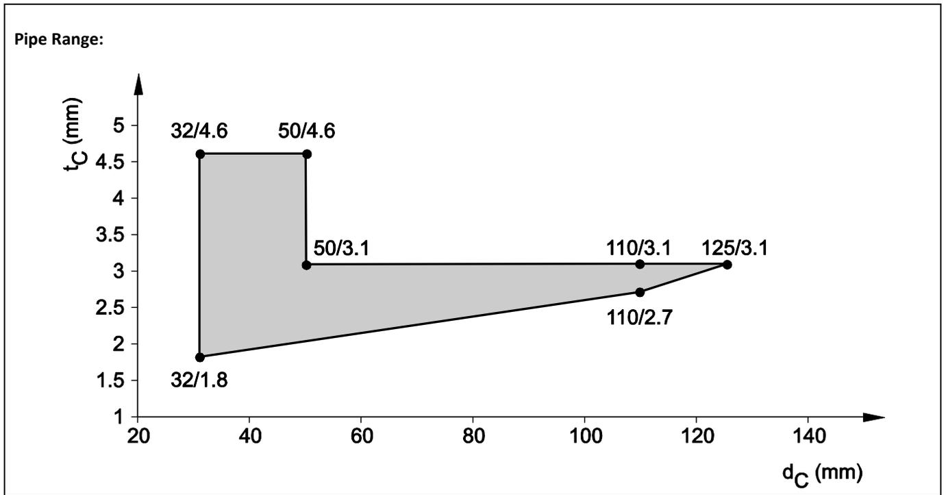
8.3.2.6 PE pipes acc. EN 15494 and EN 12201-2, in flexible wall ( $t_E \geq 100$  mm), pipe group 1, EI 120 - U/C
