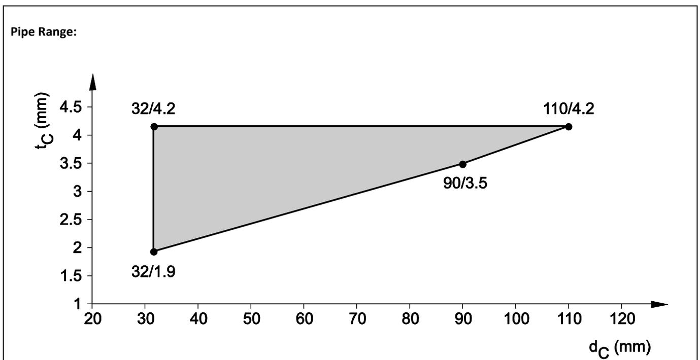
8.3.2.3 ABS- pipes acc. EN 1455, EN 15493 and SAN+PVC-pipes acc. EN 1565-1, in flexible wall, ( $t_E \geq 100$  mm), pipe group 1, EI 60 - U/U
