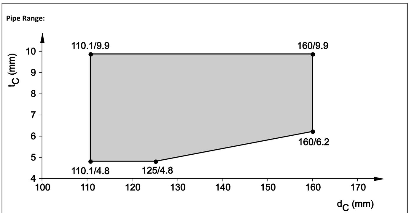
8.4.2.23 PE pipes acc. EN 15494 and EN 12201-2, in rigid wall ( $t_E \geq 150$  mm), pipe group 2, EI 120 - U/U
