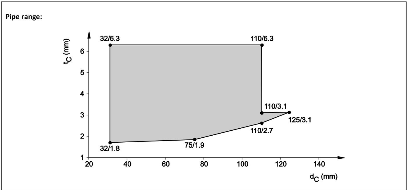
8.5.2.9 PP pipes acc. EN 1451-1, in rigid floor ( $t_E \geq 150$  mm), pipe group 1, EI 120 - U/C
