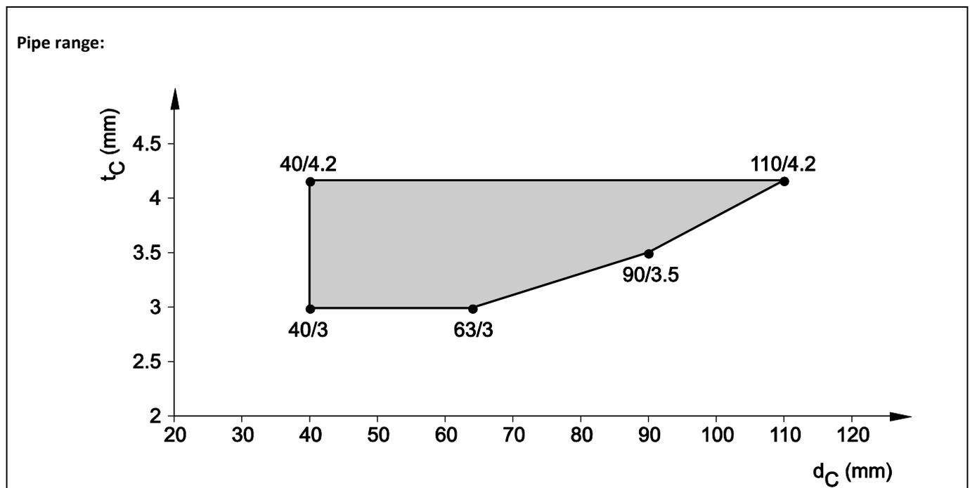
8.6.2.2 PE pipes acc. EN 15494 and EN 12201-2, in shaft wall system A, pipe group 1, EI 90 - U/U
