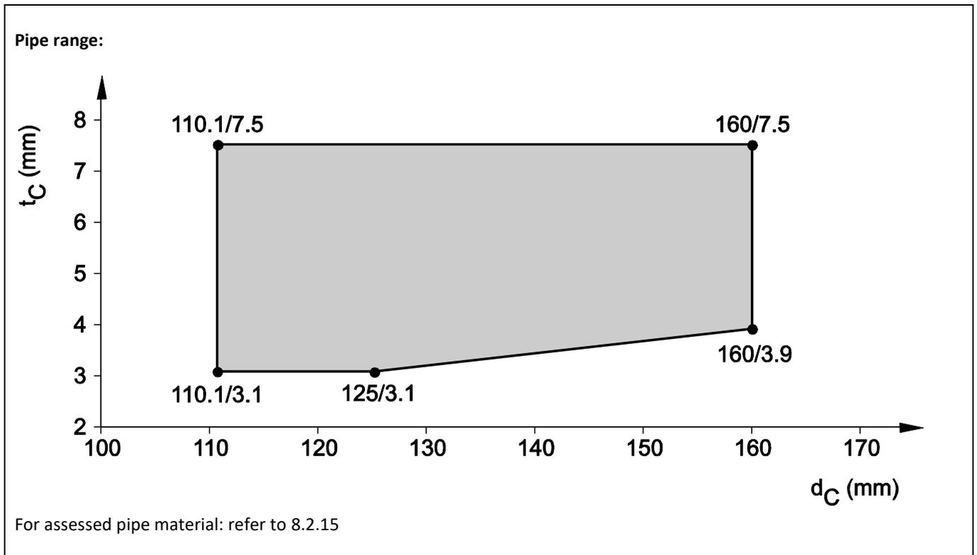
8.5.2.23 PP pipes acc. EN 1451-1, in rigid floor ( $t_E \geq 150$  mm), pipe group 2, EI 120 - U/U
