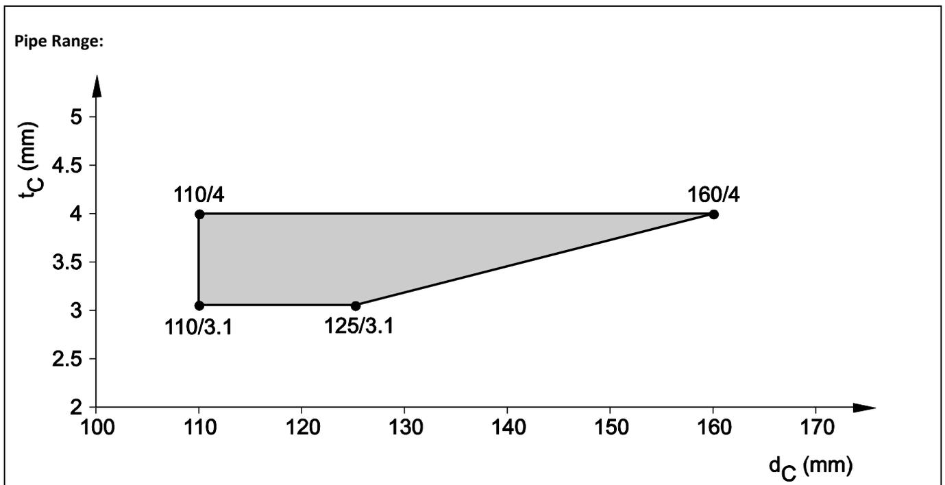
8.4.2.27 PP pipes acc. EN 1451-1, in rigid wall ( $t_E \geq 150$  mm), pipe group 2, EI 30 - U/U
