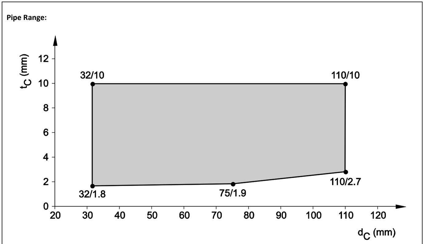
8.3.2.12 PE pipes, non-regulated (Geberit Silent dB20), in flexible wall ( $t_E \geq 100$  mm), pipe group 1, EI 120 - U/U
