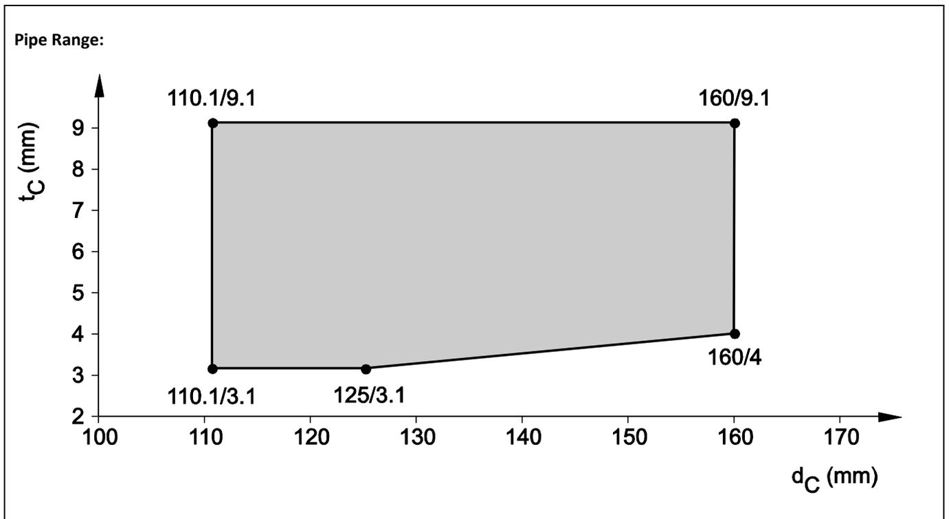
8.4.2.29 Pneumatic dispatch system, PVC pipe, in rigid wall ( $t_E \geq 150$  mm), pipe group 2, EI 90 - U/U
