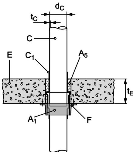
8.5.2.15 PE pipes acc. EN 1519-1, EN 12201-2 and EN 12666-1, in rigid floor ( $t_E \geq 150$  mm), pipe group 2, EI 120 - U/U
