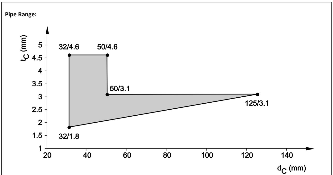
8.3.2.5 PE pipes acc. EN 15494 and EN 12201-2, in flexible wall, ( $t_E \geq 100$  mm), pipe group 1, EI 90 - U/U
