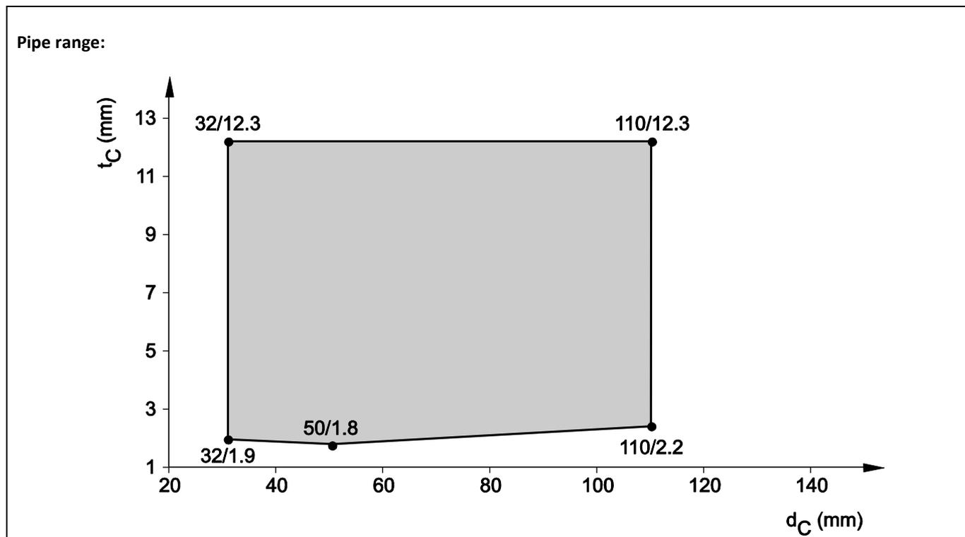
8.5.2.5 PVC pipes acc. EN 1452-1, EN 1329-1, EN 1453-1, EN 1566-1 and EN ISO 15493, in rigid floor ( $t_E \geq 150$  mm), pipe group 1, EI 90 - U/U
