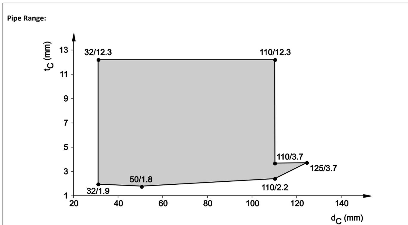
8.3.2.9 PP pipes, non-regulated in flexible wall ( $t_E \geq 100$  mm), pipe group 1, EI 90 - U/U
