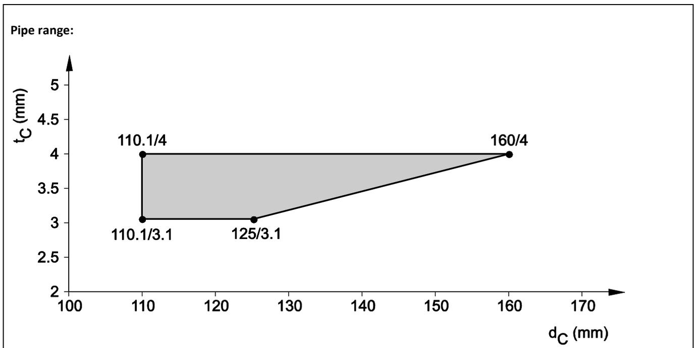
8.5.2.21 PVC pipes acc. EN 1452-1, EN 1453-1, EN 1566-1, EN 1329-1 and EN ISO 15493, in rigid floor ( $t_E \geq 150$  mm), pipe group 2, EI 90 - U/U
