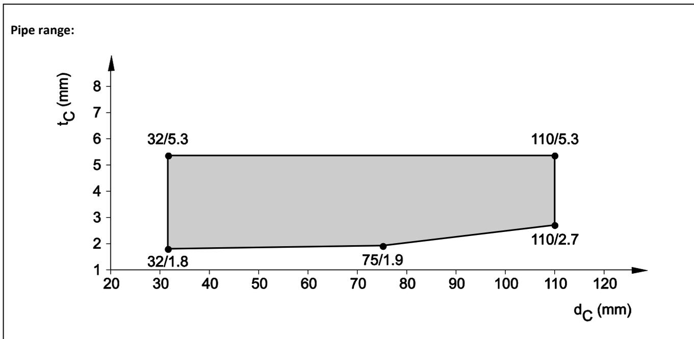
8.5.2.7 PP pipes acc. EN 1451-1, in rigid floor ( $t_E \geq 150$  mm), pipe group 1, EI 120 - U/U
