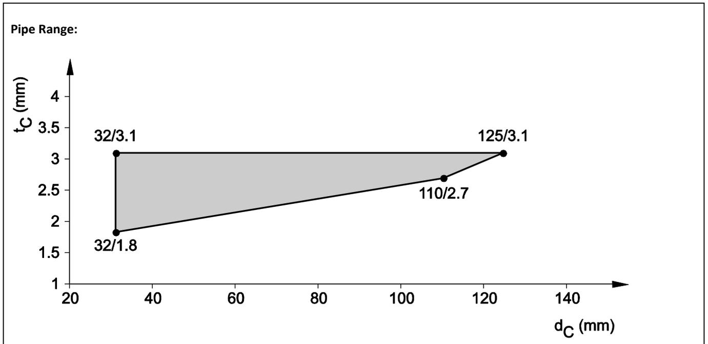
8.4.2.7 PP pipes acc. EN1451-1, in rigid wall ( $t_E \geq 100$  mm), pipe group 1, EI 120 - U/C
