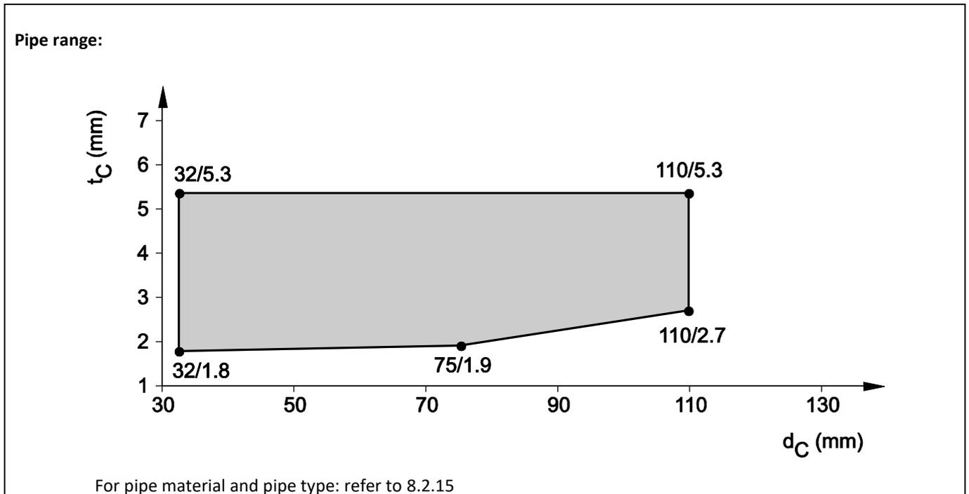
8.6.2.5 PP pipes acc. EN 1451-1, in shaft wall system A, pipe group 1, EI 90 - U/U
