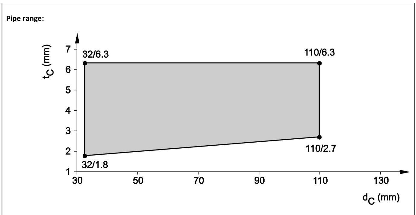
8.6.2.6 PE pipes non-regulated (Geberit Silent dB20), in shaft wall system A, pipe group 1, EI 90 - U/U
