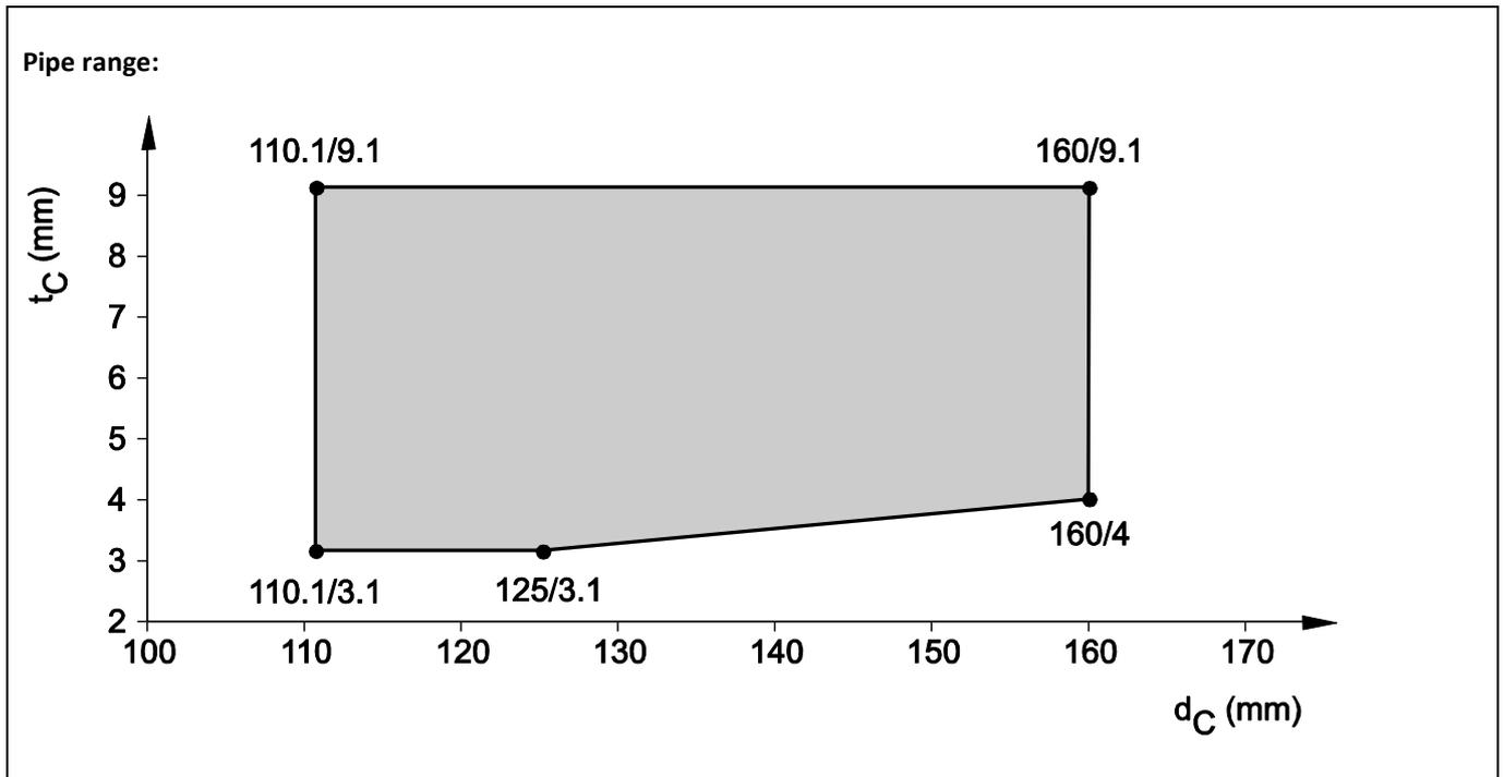
8.5.2.24 Pneumatic dispatch system, PVC-U pipes, in rigid floor ( $t_E \geq 150$  mm), pipe group 2, EI 120 - U/U, straight ( $90^\circ$ ) installed
