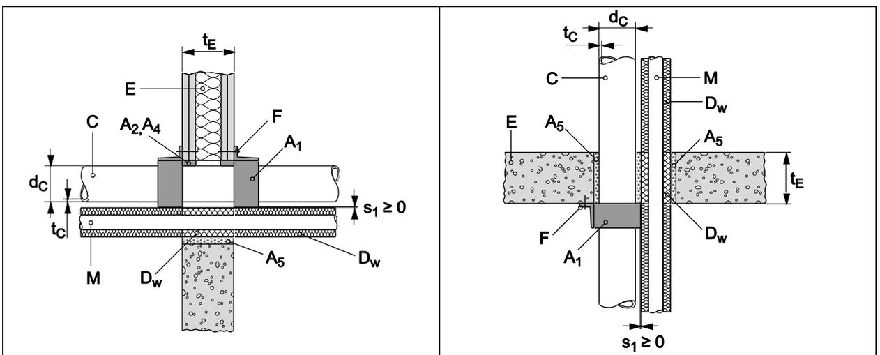
8.2.10.3 **Minimum distance Hilti Firestop Collar Endless CFS-C EL to metal pipes, aluminum composite pipes and PP-R pipes insulated with a flexible, elastomeric thermal insulation  $D_E$  and fire stopped with Hilti CFS-B**
