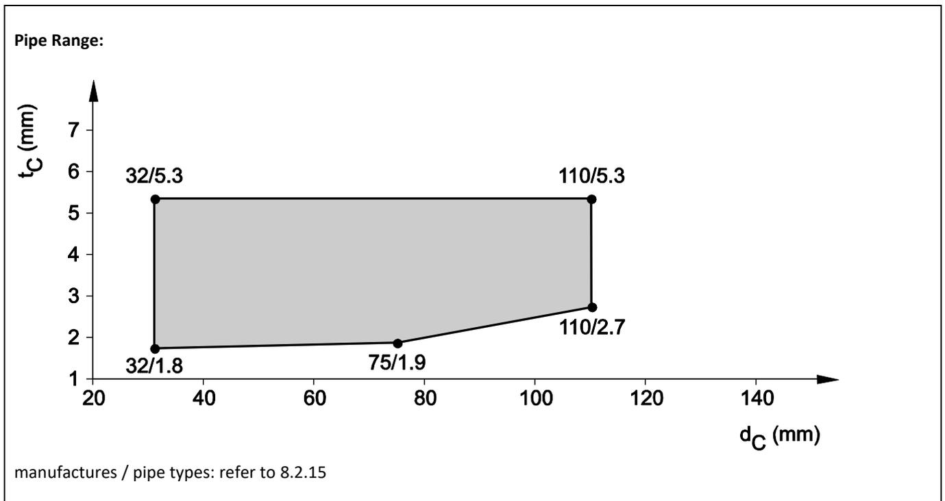
8.4.2.6 PP pipes acc. EN1451-1, in rigid wall ( $t_E \geq 100$  mm), pipe group 1, EI 120 - U/U
