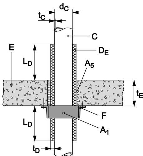
8.5.2.29 **PP-R - pipes acc. EN 15874 (Aquatherm fusiofen = aquatherm green pipe S), insulated, in rigid floor ( $t_E \geq 150$  mm), pipe group 1, EI 120 - U/C**
