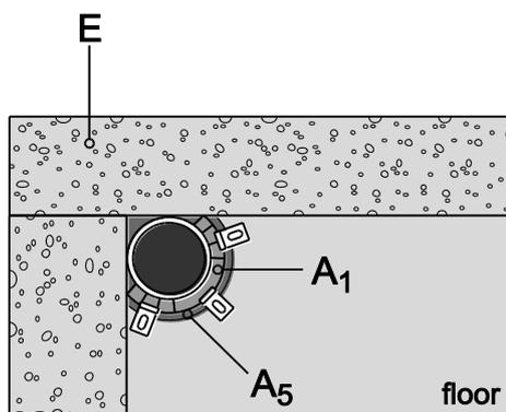
8.5.2.37 Pipes in rigid floor ( $t_E \geq 150$  mm), pipe group 1, EI 120 - U/U, pipe on wall application – zero distance to one wall when penetrating the floor
