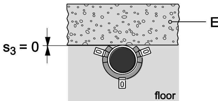
8.5.2.38 All PP pipes non-regulated, named in 8.5.2.6; in rigid floor ( $t_E \geq 150$  mm), pipe group 1, EI 120 - U/U, pipe coupling
