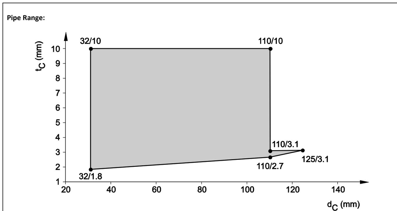
8.3.2.8 PVC pipes acc. EN 1452-1, EN 1329-1, EN 1453-1, EN 1566-1 and EN ISO 15493, in flexible wall ( $t_E \geq 100$  mm), pipe group 1, EI 120 - U/U
