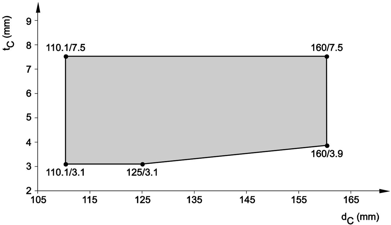
8.4.2.12 PE pipes, non-regulated (Geberit Silent dB20), in rigid wall ( $t_E \geq 100$  mm), pipe group 1, EI 120 – U/U, specific application: 2 x 45° elbow connector
