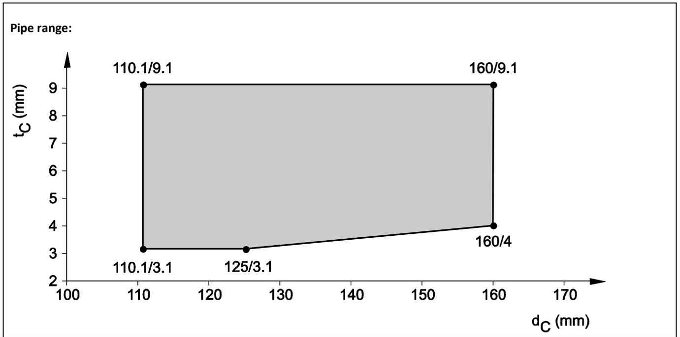
8.5.2.20 PE pipes acc. EN 15494 and EN 12201-2, in rigid floor ( $t_E \geq 150$  mm), pipe group 2, EI 120 - U/U
