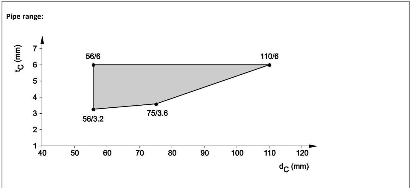
8.6.3.4 Plastic pipes, with 1x 87° elbow in shaft wall system B (refer to 8.6.1.3), EI 90 - U/U
