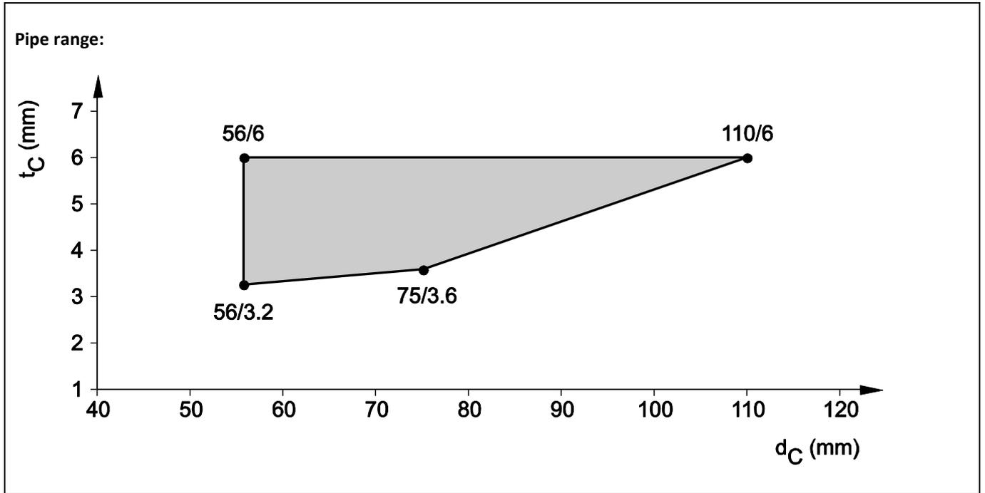
8.6.2.7 ABS pipes acc. EN 1455-1, EN 15493 and SAN+PVC-pipes acc. EN 1565-1, in shaft wall system A, pipe group 1, EI 90 - U/U
