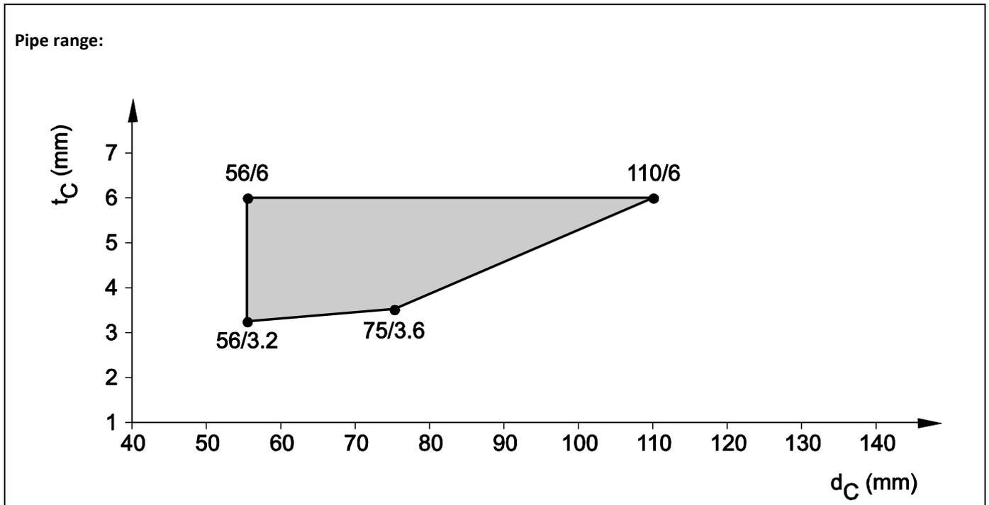
8.5.2.11 PVC-pipes, non-regulated (Friatec Friaphon), in rigid floor ( $t_E \geq 150$  mm), pipe group 1, EI 180 - U/U
