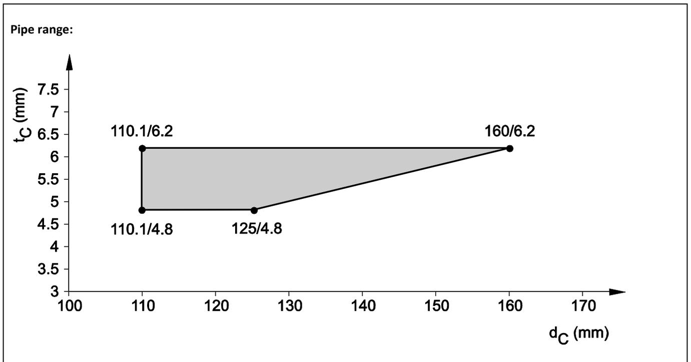
8.5.2.17 ABS pipes acc. EN 1455-1, EN 15493 and SAN+PVC-pipes acc. EN 1565-1, in rigid floor ( $t_E \geq 150$  mm), pipe group 2, EI 60 - U/U
