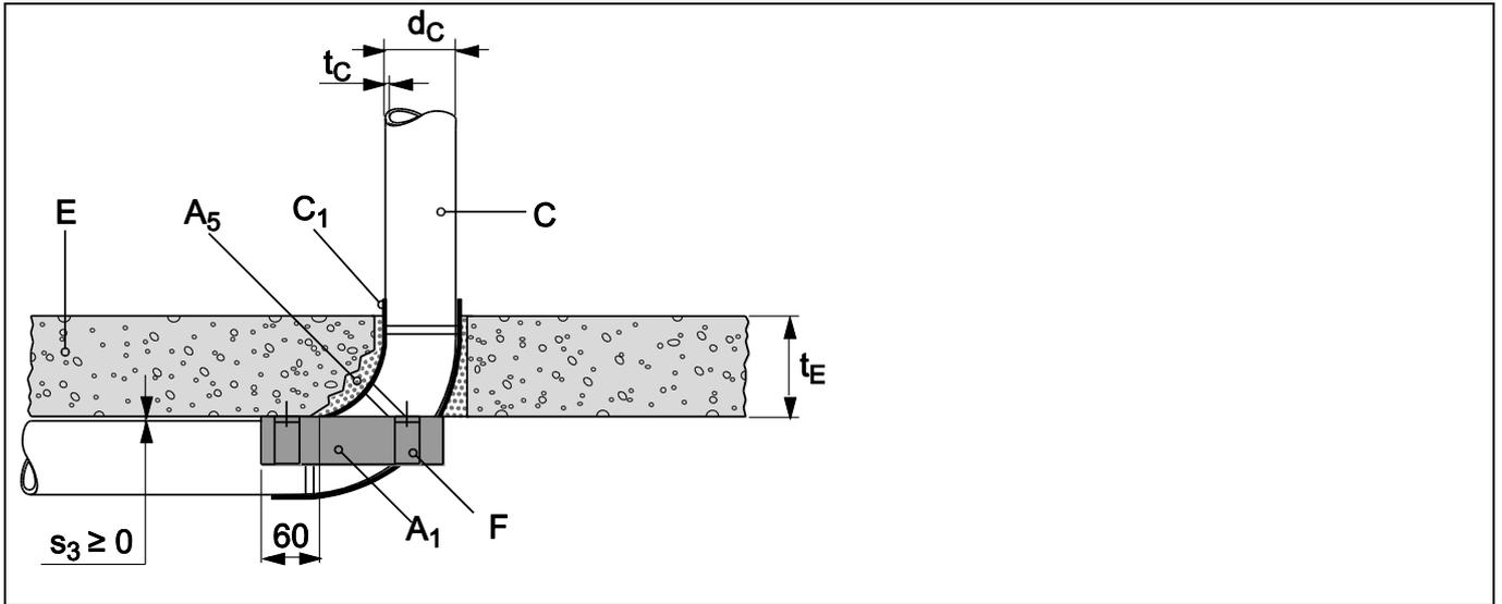
8.5.2.14 PE pipes, non-regulated (Geberit Silent dB20), in rigid floor ( $t_E \geq 150$  mm), pipe group 1, EI 120 - U/U straight (90°), pipe coupling
