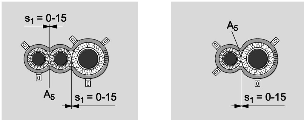
**8.5.2.31 Reuse of oddments of CFS-C EL, in rigid floor ( $t_e \geq 150 \text{ mm}$ ), pipe group 1 and 2, EI 120 - U/U**
