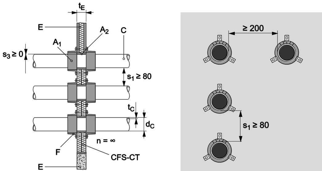
8.3.2.25 Pipes in flexible wall ( $t_E \geq 100$  mm), pipe group 1, EI 90 - U/U, CFS-C EL collar to collar (zero distance)
