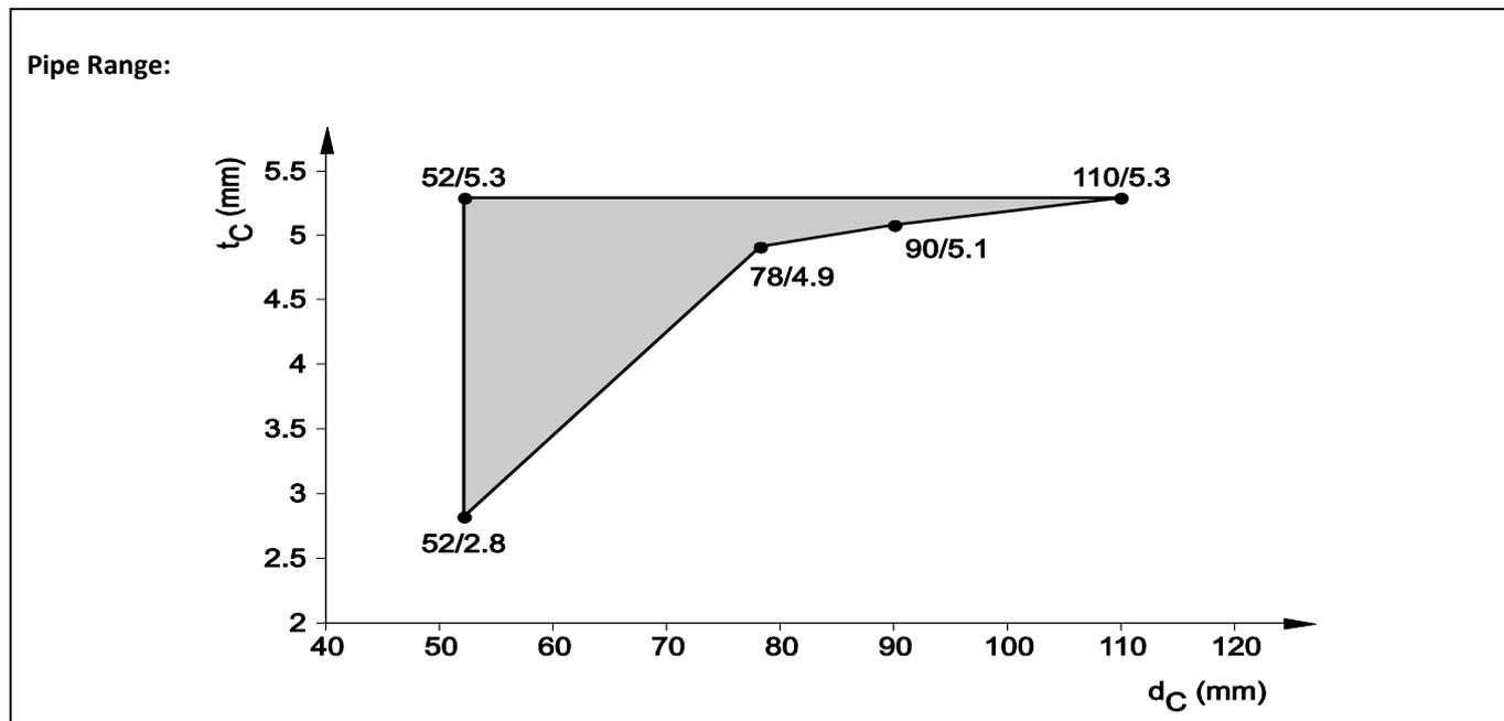
8.3.2.14 Pneumatic dispatch system, PVC pipe, in flexible wall ( $t_E \geq 100$  mm), pipe group 1, EI 90 - U/U
