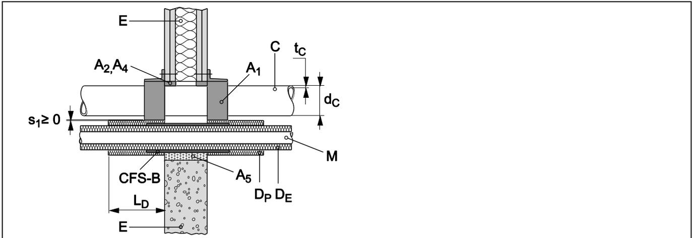
**8.3.2.23.2 Pipes in flexible wall ( $t_E \geq 100$  mm), pipe group 1, EI 90, zero distance between CFS-C EL collar and CFS-B, wrapped around an elastomeric foamed thermal insulation on metal pipe**
