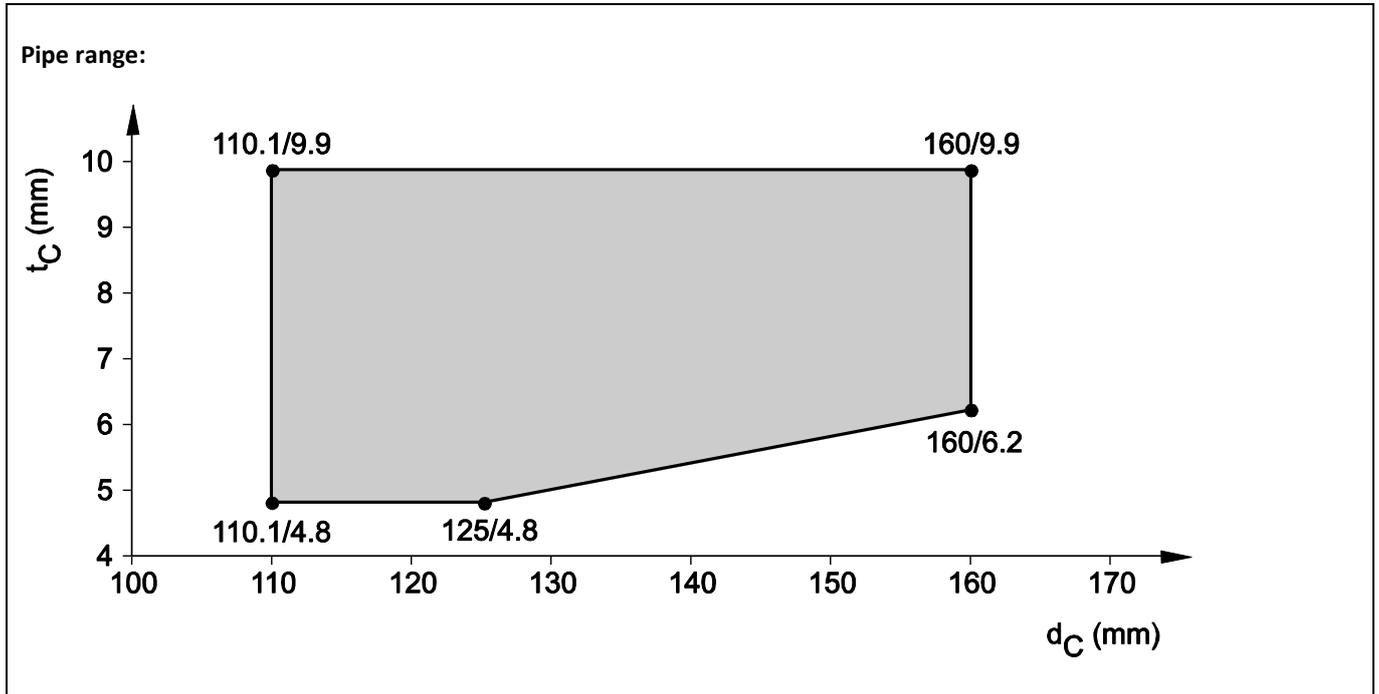
8.5.2.18 PE pipes acc. EN 15494 and EN 12201-2, in rigid floor ( $t_E \geq 150$  mm), pipe group 2, EI 90 - U/U
