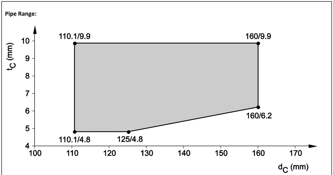
8.4.2.22 ABS pipes acc. EN 1455-1, EN 15493 and SAN+PVC-pipes acc. EN 1565-1, in rigid wall ( $t_E \geq 150$  mm), pipe group 2, EI 120 - U/C
