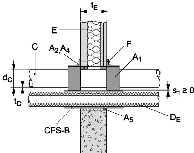
PE foamed insulation or PE protection tube on aluminum composite EI90 U/C
