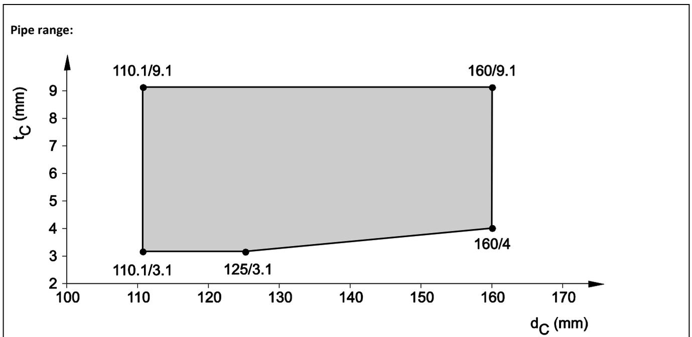
8.5.2.19 PE pipes acc. EN 15494 and EN 12201-2, in rigid floor ( $t_E \geq 150$  mm), pipe group 2, EI 120 - U/C
