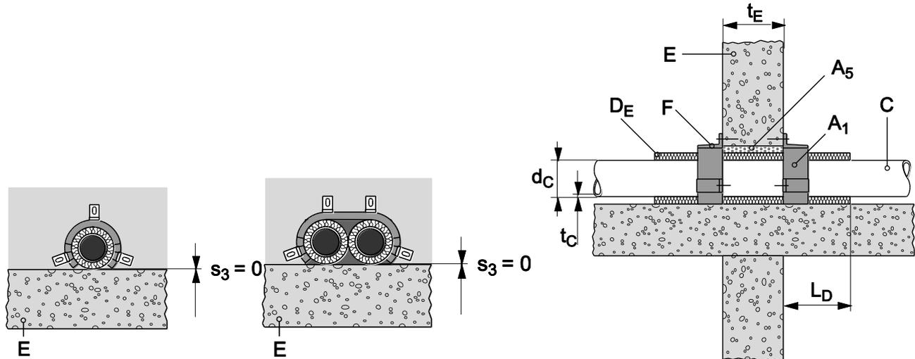
8.4.2.11 **Roof drainage, covered with foamed elastomeric thermal insulation, in rigid wall**
