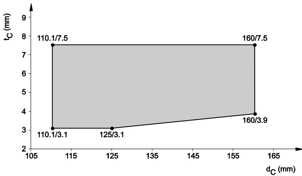
8.5.2.45 Pipe junction/manifold inside the floor, assessed in rigid floor ( $t_E \geq 150$  mm), pipe group 1 and 2, EI 120 - U/U, EI 90 - U/U and EI 60 - U/U
