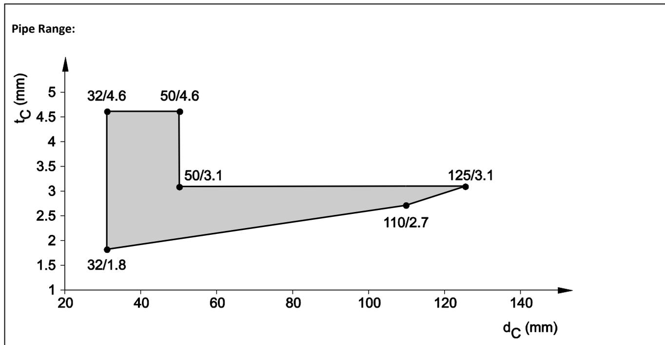
8.4.2.3 PE pipes acc. EN15494 and EN 12201-2, in rigid wall ( $t_E \geq 100$  mm), pipe group 1, EI 120 - U/C
