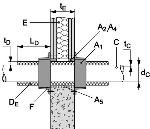
8.3.2.17 PP pipes, non-regulated, in flexible wall ( $t_E \geq 100$  mm), pipe group 1, EI 120 - U/U, Pipe coupling
