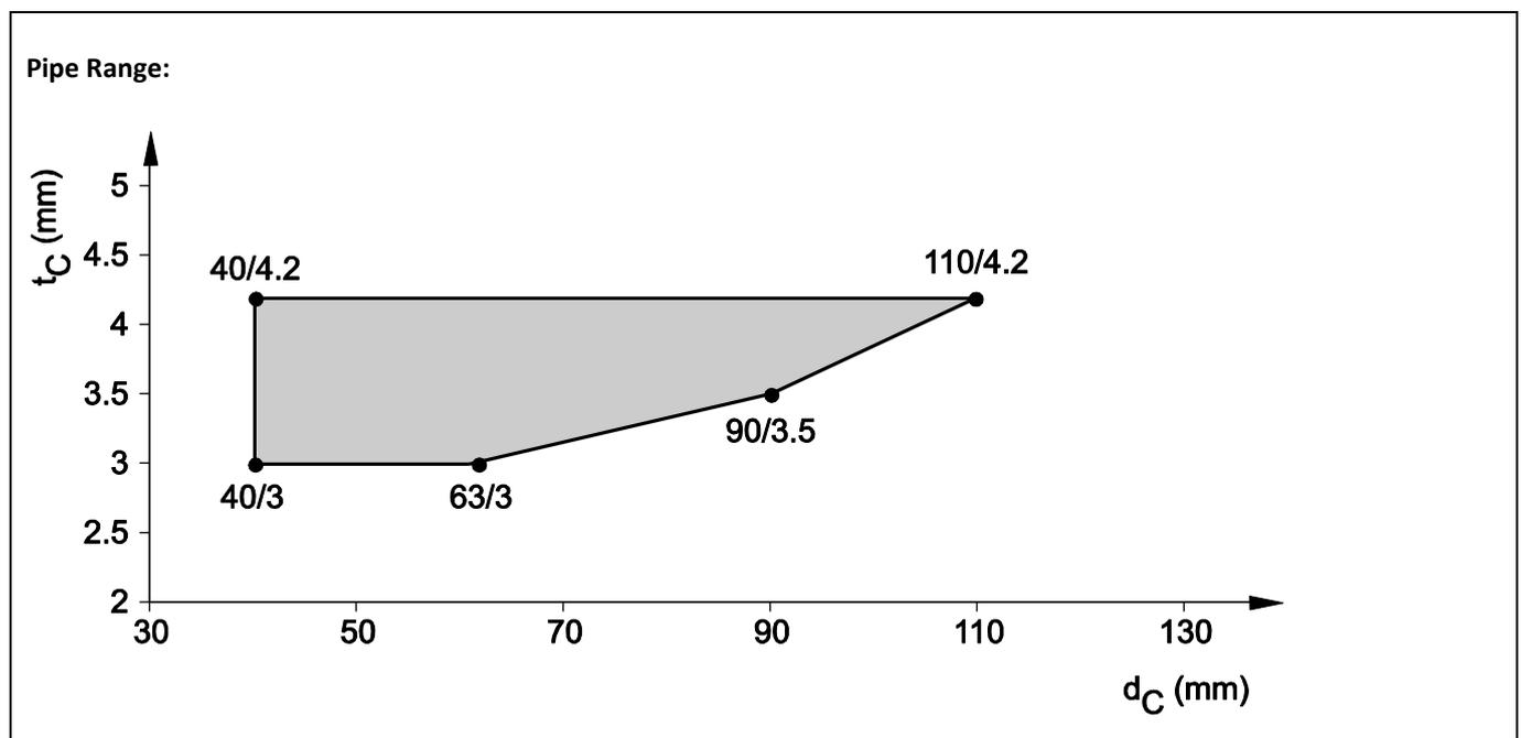
8.4.2.2 PE pipes acc. EN15494 and EN 12201-2, in rigid wall ( $t_E \geq 100$  mm), pipe group 1, EI 120, U/U
