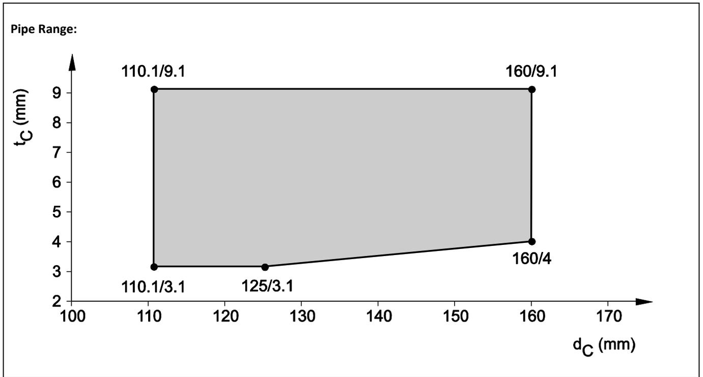
8.4.2.24 PVC pipes acc. EN 1452-1, EN 1329-1, EN 1453-1, EN1566-1 and EN ISO 15493, in rigid wall ( $t_E \geq 150$  mm), pipe group 2, EI 120 - U/U
