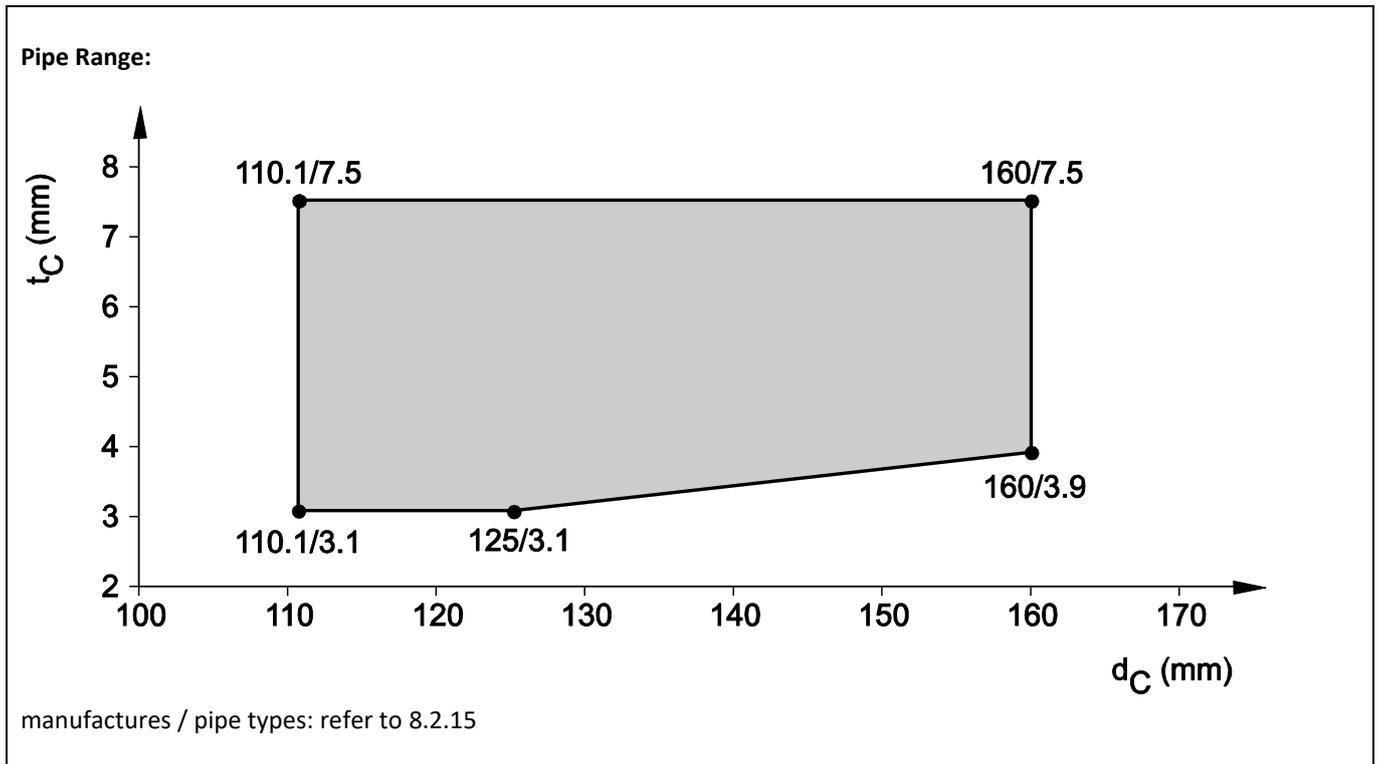
8.4.2.26 PP pipes acc. EN 1451-1, in rigid wall ( $t_E \geq 150$  mm), pipe group 2, EI 120 - U/U
