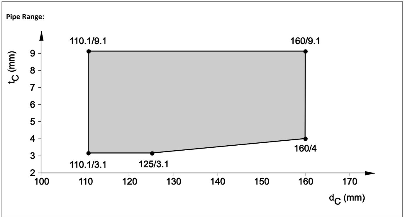
8.4.2.28 PP pipes acc. EN 1451-1, in rigid wall ( $t_E \geq 150$  mm), pipe group 2, EI 120 - U/C
