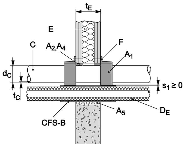
Aluminum composite pipes EI60 U/C
