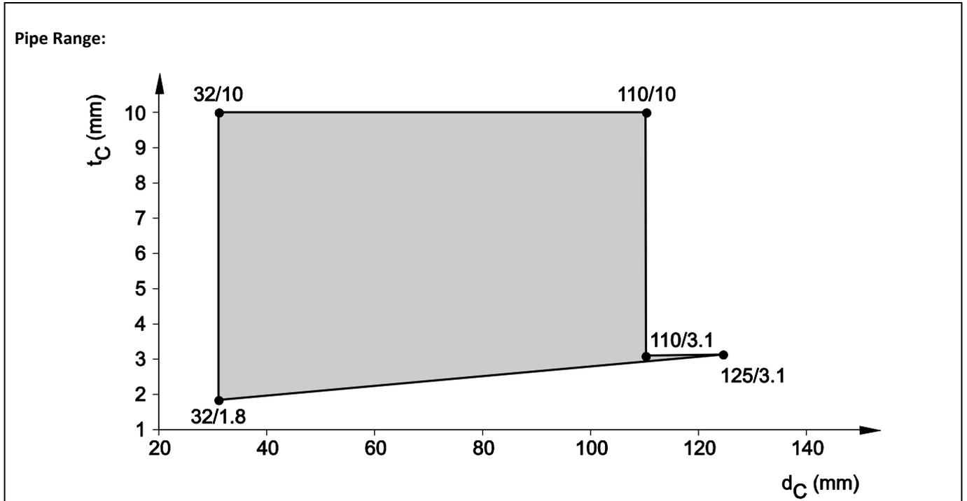
8.3.2.7 PE pipes acc. EN 15494 and EN 12201-2, in flexible wall ( $t_E \geq 100$  mm), pipe group 1, EI 90 - U/C
