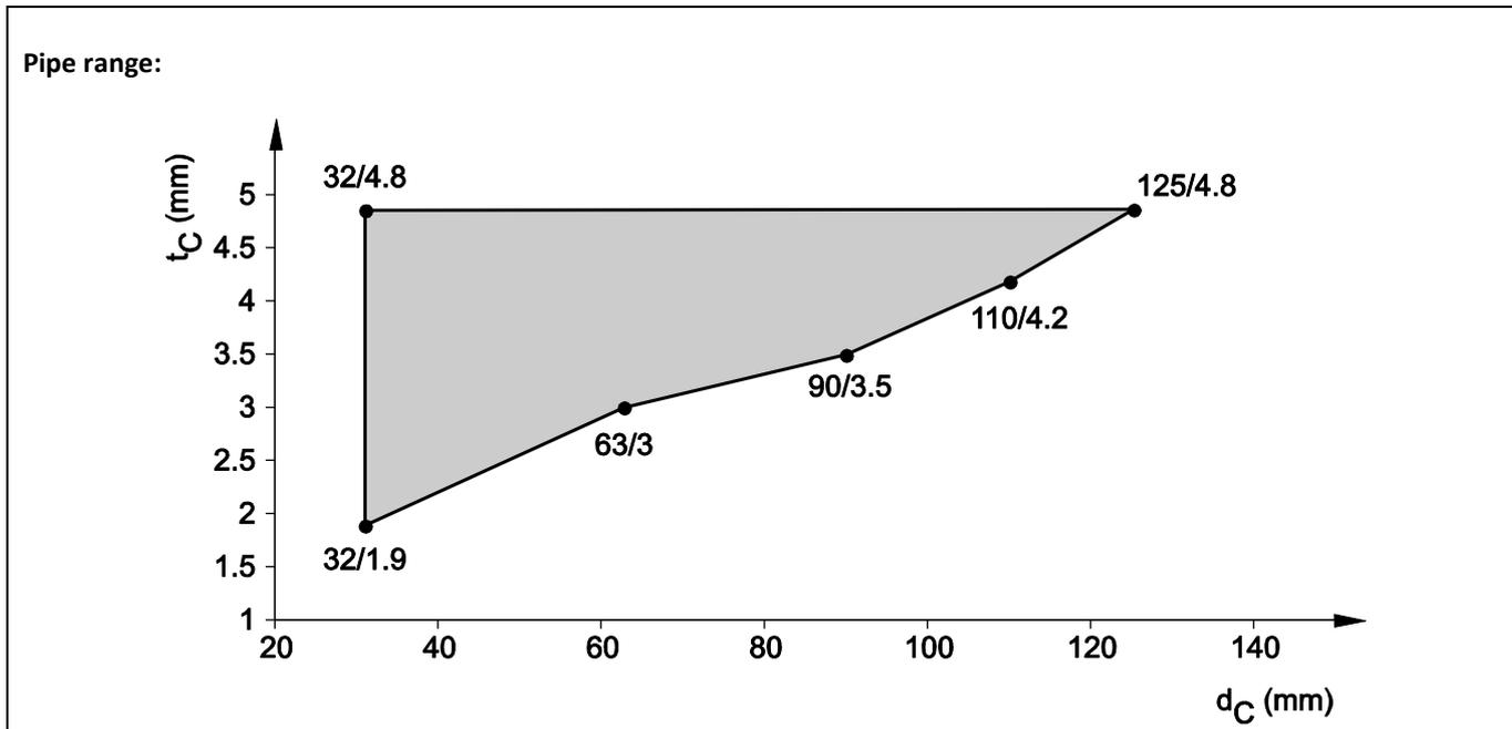
8.5.2.3 PE pipes acc. EN 15494 and EN 12201-2, in rigid floor ( $t_E \geq 150$  mm), pipe group 1, EI 120 - U/U
