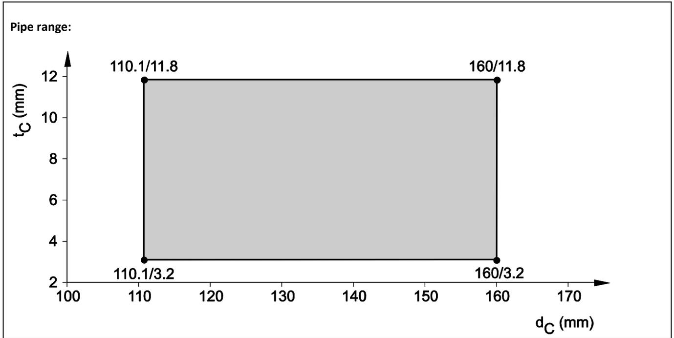
8.5.2.22 PP pipes, non-regulated, in rigid floor ( $t_E \geq 150$  mm), pipe group 2, EI 120 - U/U
