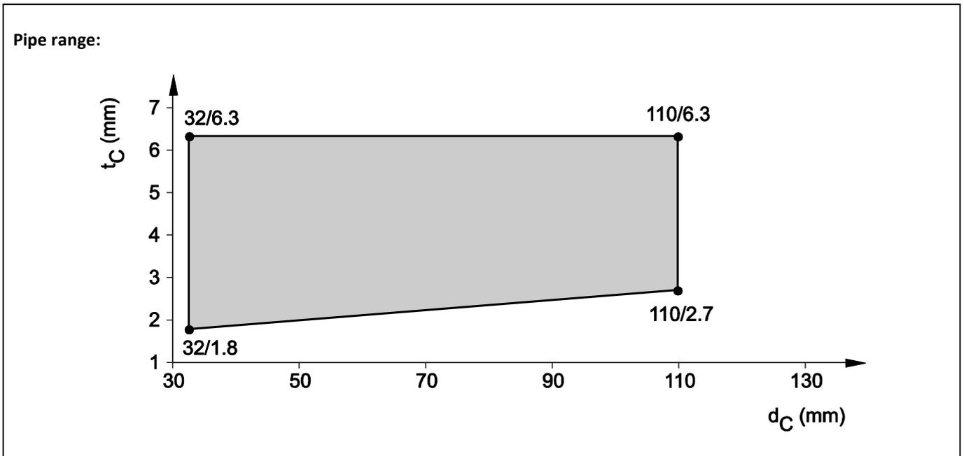
8.6.2.3 PVC pipes acc. EN 1452-1, EN 1329-1, EN 1453-1, EN 1566-1 and EN ISO 15493, in shaft wall system A, pipe group 1, EI 90 - U/U
