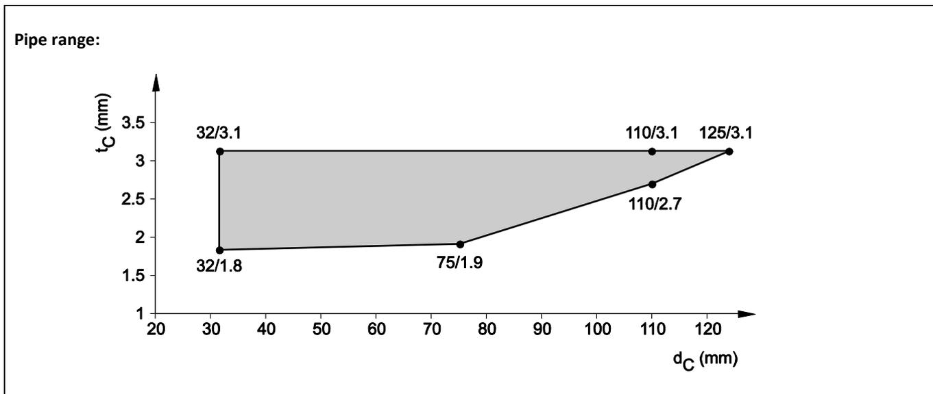
8.5.2.8 PP pipes acc. EN 1451-1, in rigid floor ( $t_E \geq 150$  mm), pipe group 1, EI 90 - U/U
