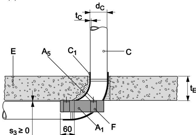
8.5.2.36 Pipes in rigid floor ( $t_f \geq 150$  mm), pipe group 1, EI 90 - U/U, pipe in corner application – zero distance to two walls
