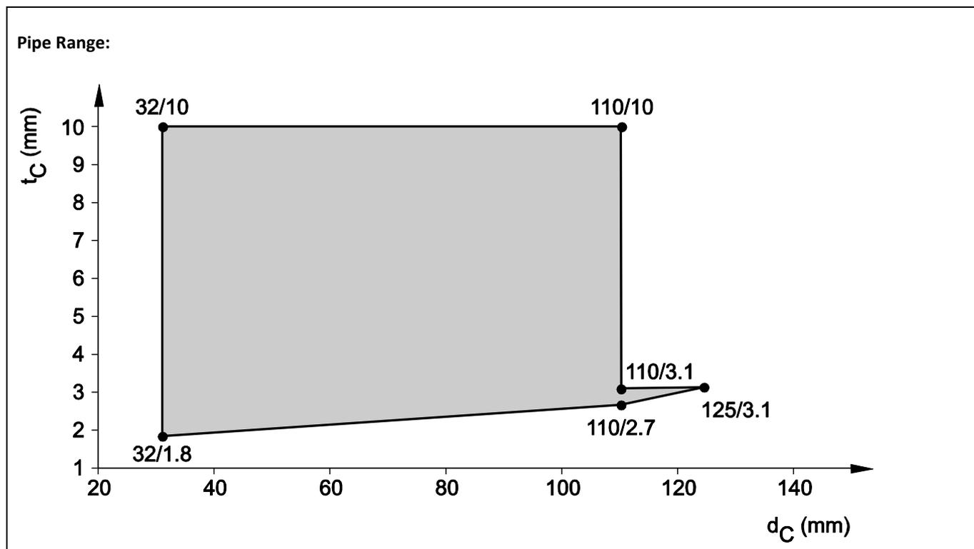
8.4.2.4 PVC pipes acc. EN 1452-1, EN 1329-1, EN 1453-1, EN1566-1 and EN ISO 15493, in rigid wall ( $t_E \geq 100$  mm), pipe group 1, EI 120 - U/U
