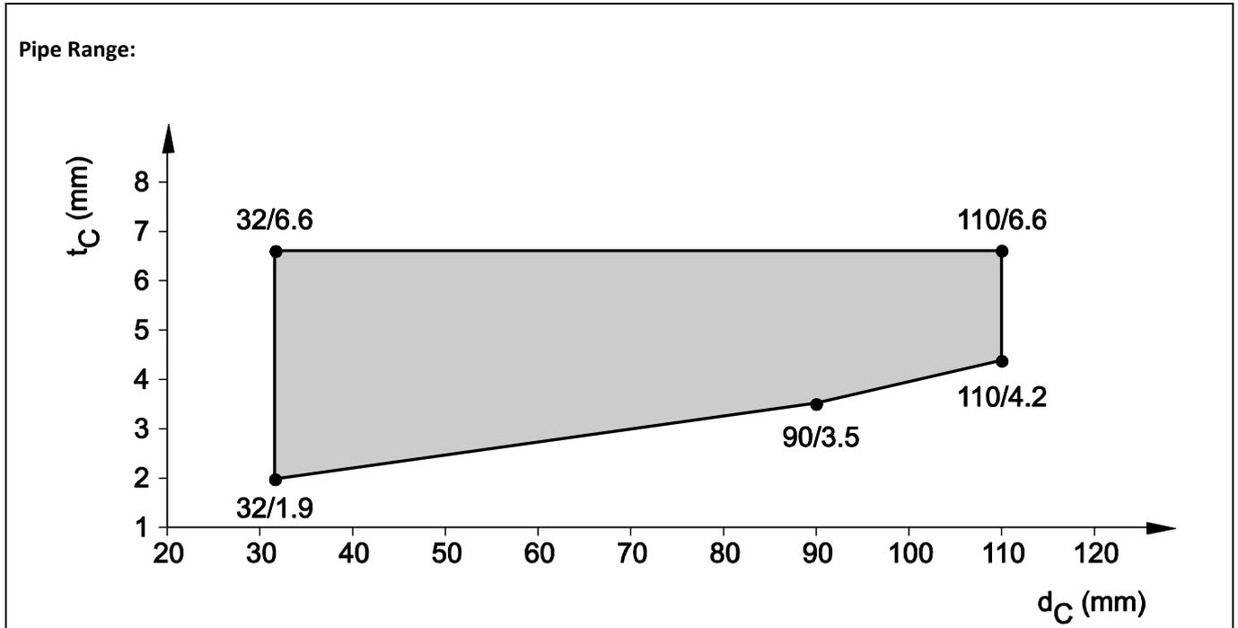
8.3.2.4 PE pipes acc. EN 15494 and EN 12201-2, in flexible wall, ( $t_E \geq 100$  mm), pipe group 1, EI 120 - U/U
