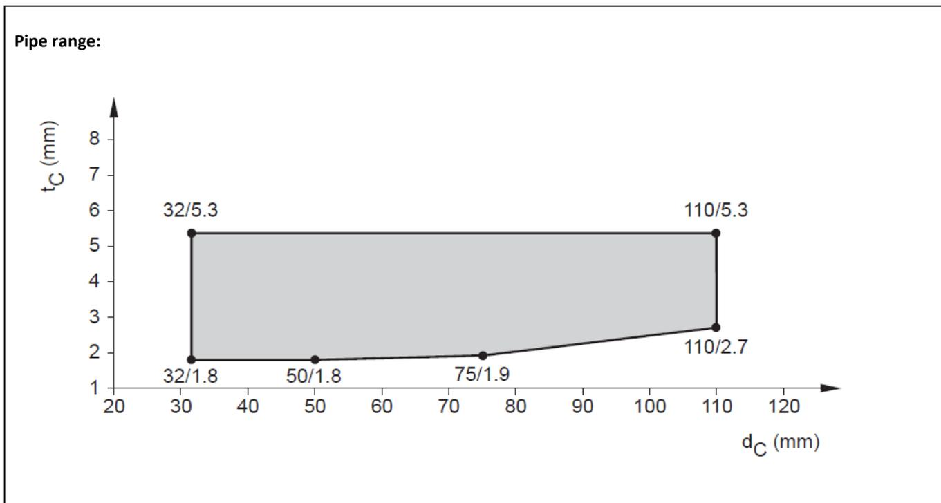
8.6.3.3 PE pipes, non-regulated (Geberit Silent dB20) in shaft wall system B, pipe group 2, EI 90 - U/U
