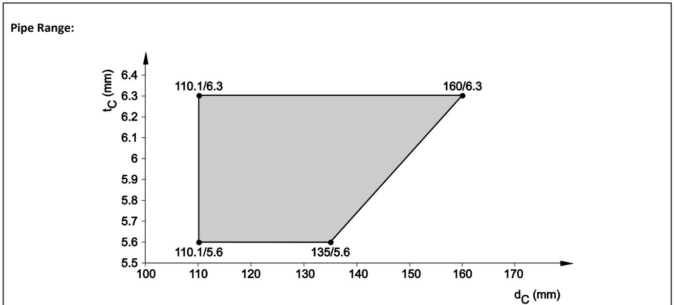
8.5.2.28 PE-X - pipes acc. EN 15875 (Rehau Rautitan flex), insulated, in rigid floor ( $t_E \geq 150$  mm), pipe group 1, EI 120 - U/C
