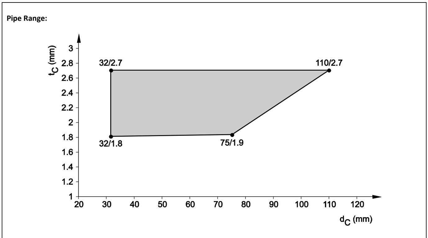
8.3.2.11 PP pipes acc. EN 1451-1, in flexible wall ( $t_E \geq 100$  mm), pipe group 1, EI 120 - U/C
