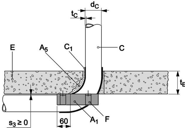
**8.5.2.48 PVC pipes acc. EN 1452-1, EN 1329-1, EN 1453-1, EN 1566-1 and EN ISO 15493, in rigid floor ( $t_E \geq 150$  mm), pipe group 1, EI 120 - U/U, Pipe Elbow 87°**
