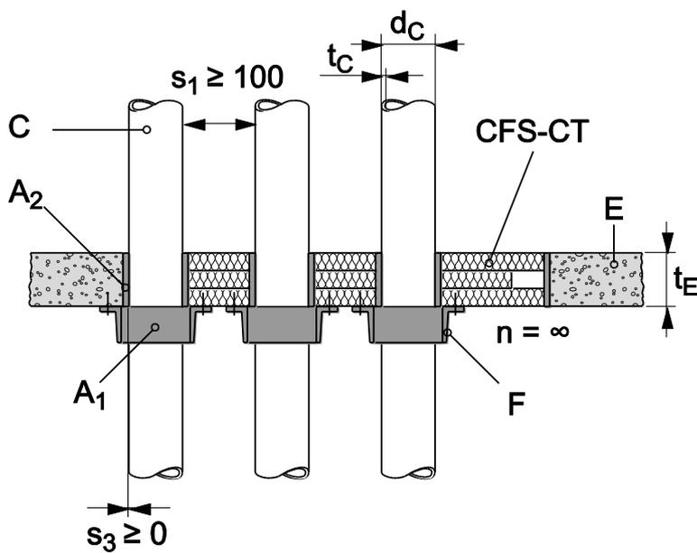
8.5.2.44 **Roof drainage covered with foamed elastomeric thermal insulation in rigid floor**
