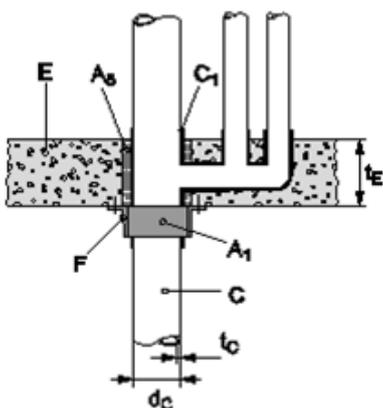
8.5.2.46 PP pipes acc. EN 1451-1, in rigid floor ( $t_E \geq 150$  mm), pipe group 1, EI 120 - U/U, Pipe coupling
