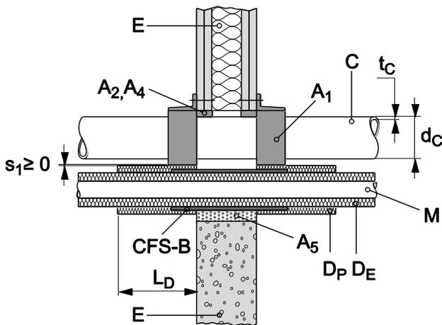
8.3.2.23.3 Pipes in flexible wall ( $t_E \geq 100$  mm), pipe group 1, EI 60/90, zero distance between CFS-C EL collar and CFS-B, wrapped around an elastomeric foamed thermal insulation on aluminium composite and PP-R pipes
