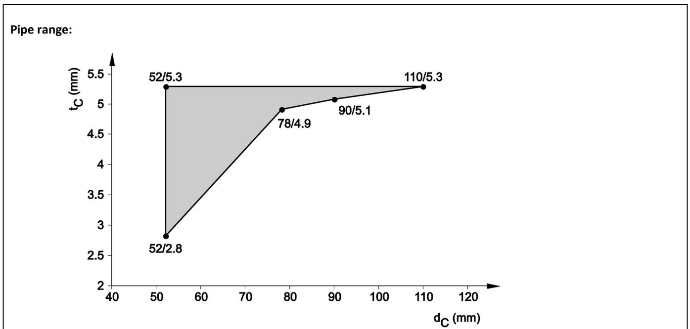
8.5.2.12 **Pneumatic dispatch system, PVC-U pipes, in rigid floor ( $t_E \geq 150$  mm), pipe group 1, EI 120 - U/U, Pipe inclination: ( $45^\circ \leq$  pipe inclination  $\leq 90^\circ$ )**
