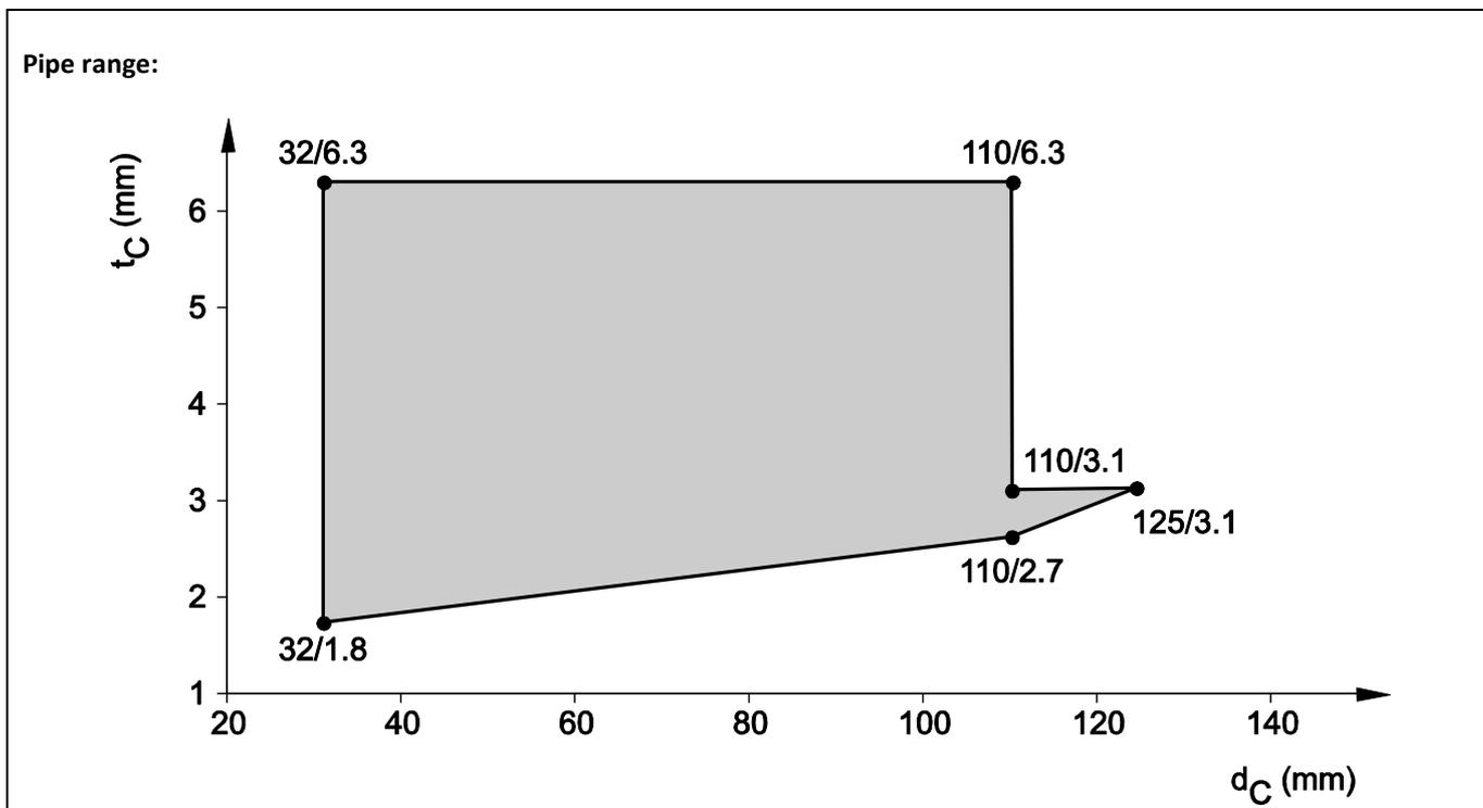
8.5.2.4 PVC pipes acc. EN 1452-1, EN 1329-1, EN 1453-1, EN 1566-1 and EN ISO 15493, in rigid floor ( $t_E \geq 150$  mm), pipe group 1, EI 120 - U/U
