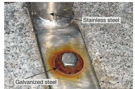
This is a typical case of contact corrosion. Zinc-plated carbon steel (washer) and stainless steel (screw and part) were used together. The surface area of the more noble metal – the stainless steel – is larger, causing strong corrosion of the washer.
