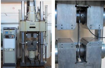
Test facility for fatigue test
