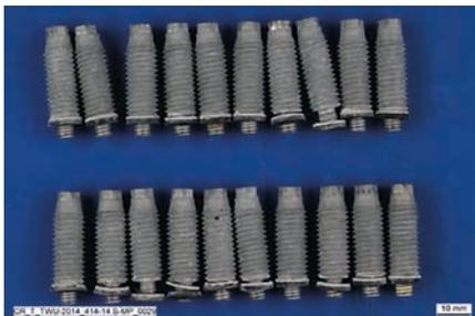
Removed S-BT fasteners after 12 weeks EN ISO 16701 cyclic corrosion test. No visible corrosion.
