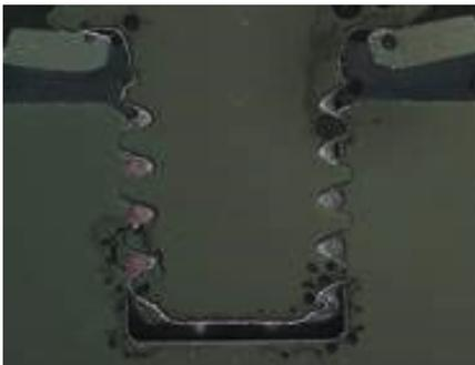
Polished cut image: activated Micro encapsulation on the tapping thread of the S-BT fastener
