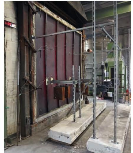
Figure 1: Test facility for fire test (big bulkhead)
